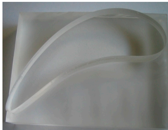
Figure 4. The shape of airfoil manufactured by Computer Numerically Controlled (CNC) machining.
