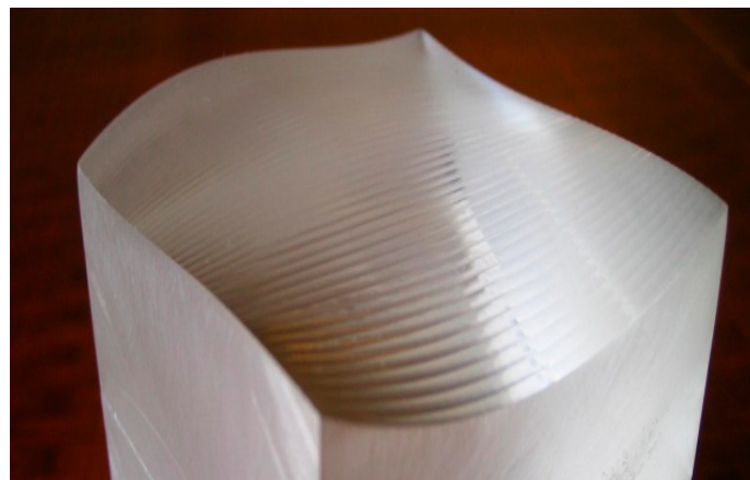
Figure 9. Manufactured freeform surface using CNC machining.
