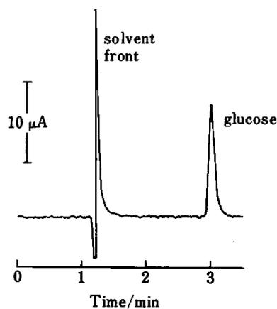
Fig. 3 Chromatograms of 1 nmol glucose in water with the Ni-MCH detector: potential, +0.45 V vs. Ag/AgCl; column, Dionex AS-7 anion exchange column; mobile phase, 0.15 M NaOH; flow rate, 1.0 ml/min.
