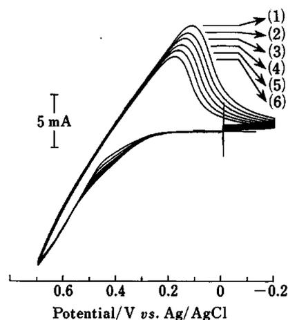
Fig. 2 Voltammetric responses of the nickel-coated hollow-fiber electrode at a scan rate of 100 mV/s in the absence (1) and presence of 1 (2), 2 (3), 3 (4), 4 (5) and 5 (6) mM of glucose in 0.15 M NaOH.
