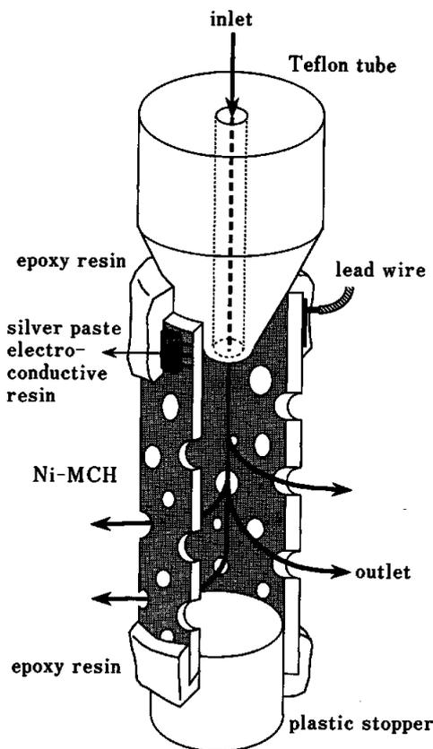
Fig. 1 Schematic representation of the nickel-coated hollow-fiber electrode for HPLC.
