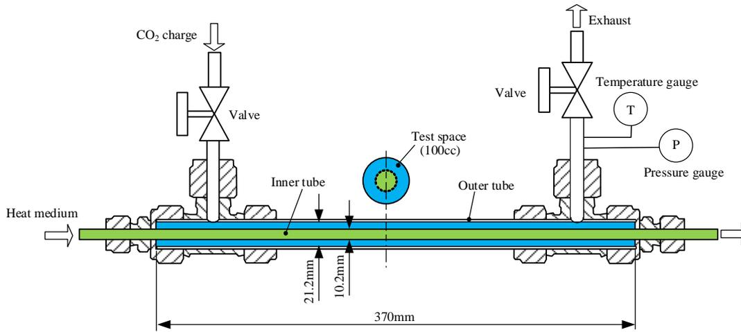
(a) Test heat exchanger
