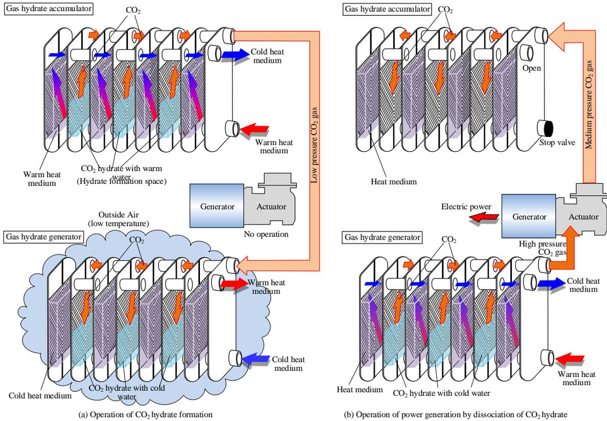
Fig. 6 Gas hydrate battery system
