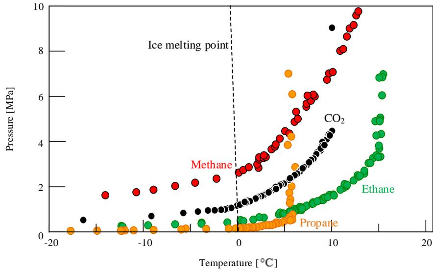
Fig. 2 Phase diagram of various kinds of gas hydrates
