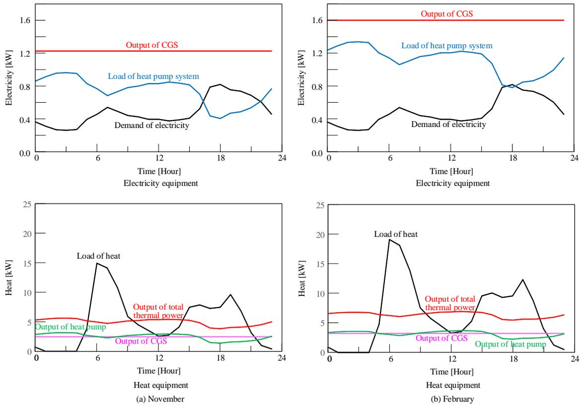
Fig. 12 Analysis results of power equipment operation for the conventional system
