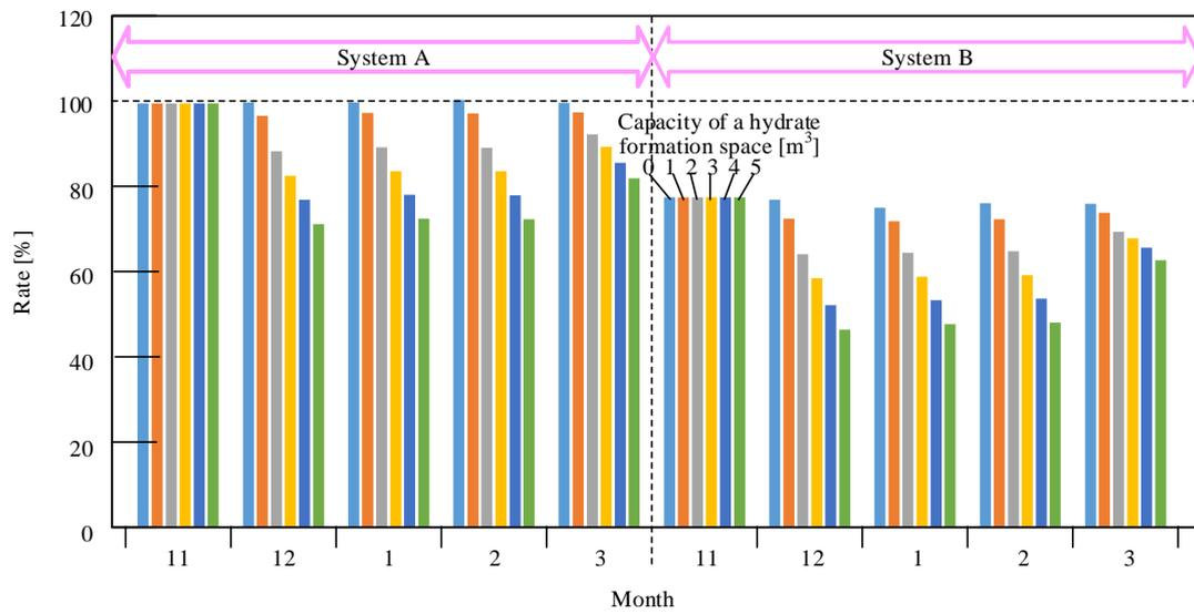
(b) Fuel consumption to the conventional system of each system
