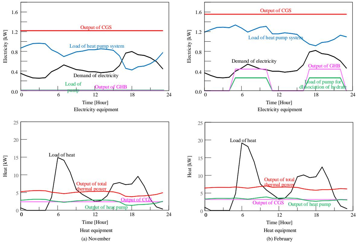
Fig. 13 Analysis results of power equipment operation for System A with hydrate formation space  $1\text{m}^3$
