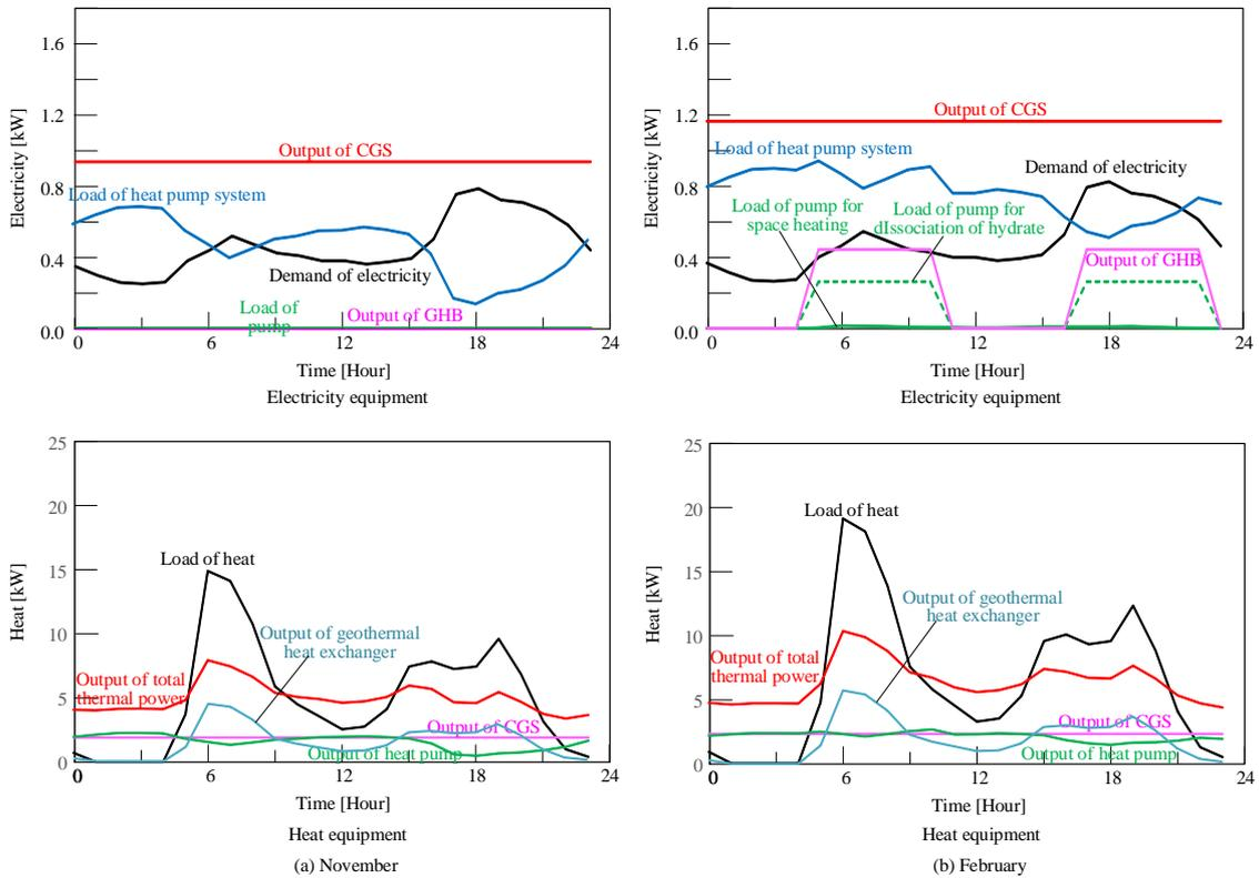
Fig. 14 Analysis results of power equipment operation for System B with hydrate formation space  $1\text{m}^3$
