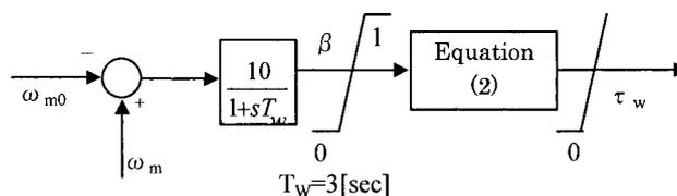
Fig. 5. Pitch control system model
