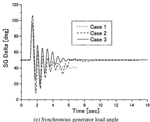
(e) Synchronous generator load angle
