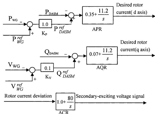
Fig. 4. Control signal blocks for DASM
