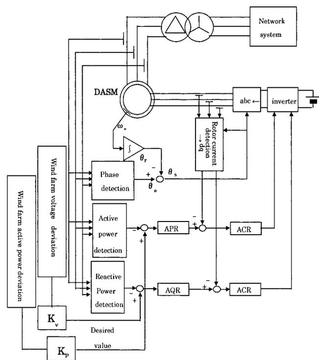
Fig. 3. DASM circuit configuration
