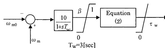
Fig. 5. Pitch control system model
