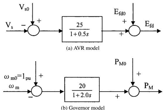
Fig. 2. Control system models of synchronous generator
