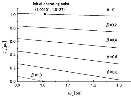
Fig. 6. Wind turbine torque characteristic
