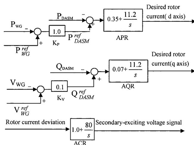
Fig. 4. Control signal blocks for DASM
