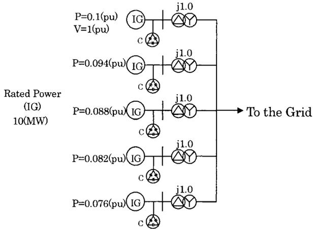
Fig. 9. Wind generator part of the model system
