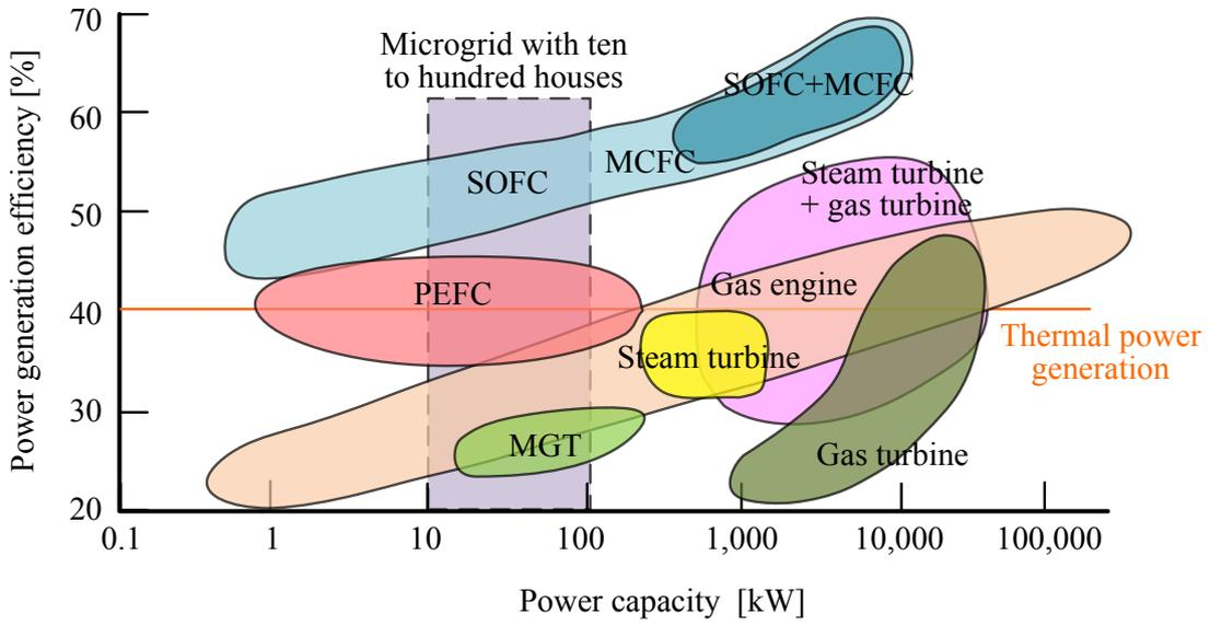
Fig. 1 Power capacity and efficiency of the power system
