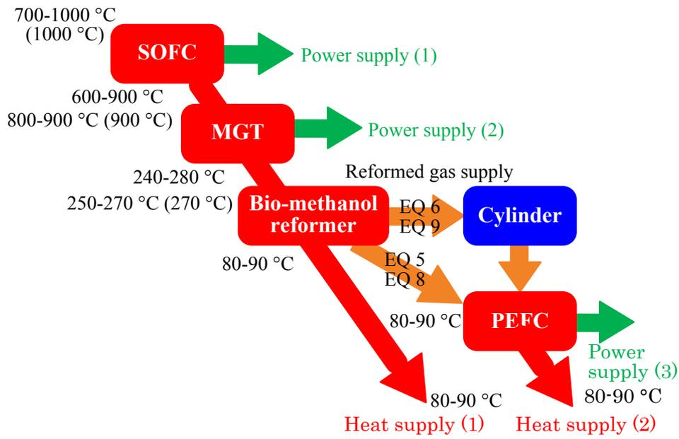
Fig. 3 Fuel cell cascade system
