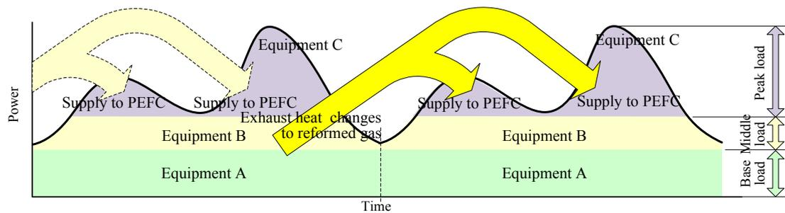
(e) Three types of equipment in a combined cascade system with time shift utilization of reformed gas
