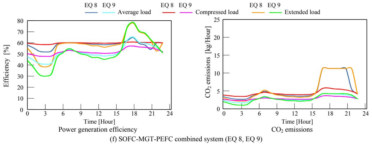
Fig. 8 Analysis results for the power generation efficiency and the CO<sub>2</sub> emissions of each piece of equipment under three load patterns
