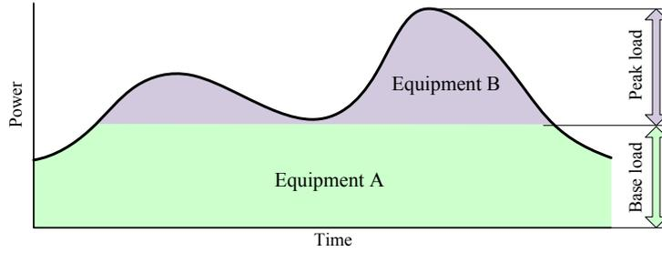
(b) Two types of equipment in a combined cascade system
