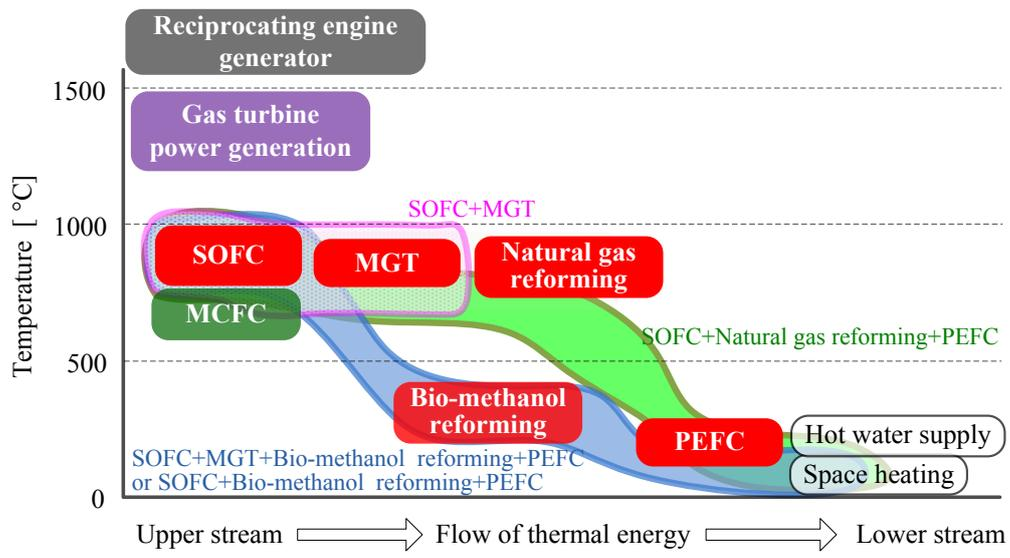
Fig. 2 Cascade system introduced into a microgrid with 100 houses
