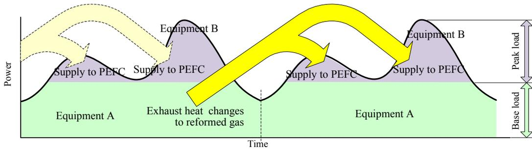
(c) Two types of equipment in a combined cascade system with time shift utilization of reformed gas
