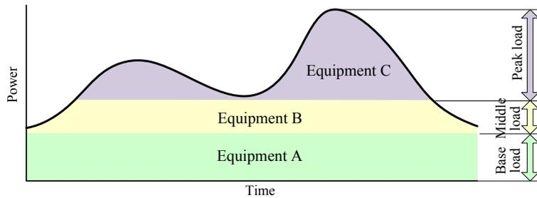
(d) Three types of equipment in a combined cascade system
