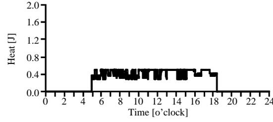
(c) Exhaust heat of the gas cooler in one minute intervals
