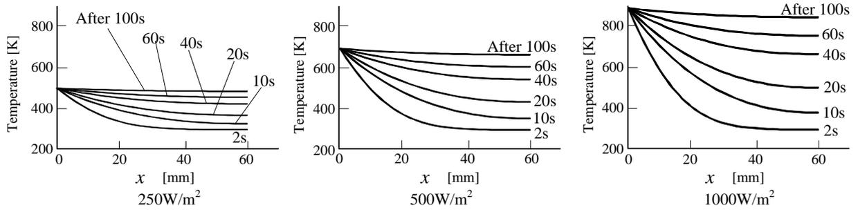
Fig. 4 Temperature distribution in the catalyst layer of the reactor
