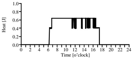
(b) Exhaust heat of the CO oxidation unit in one minute intervals
