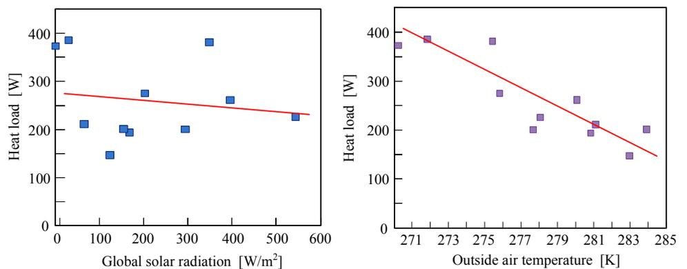
Fig. 4 Experimental result of the heat load on a model room. Heating value Required to raise the room temperature to 293 K.
