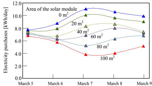
Fig. 13 Relation between the area of a solar cell and commercial-electric-power consumption
