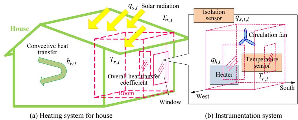
Fig. 3 Heating system and room model
