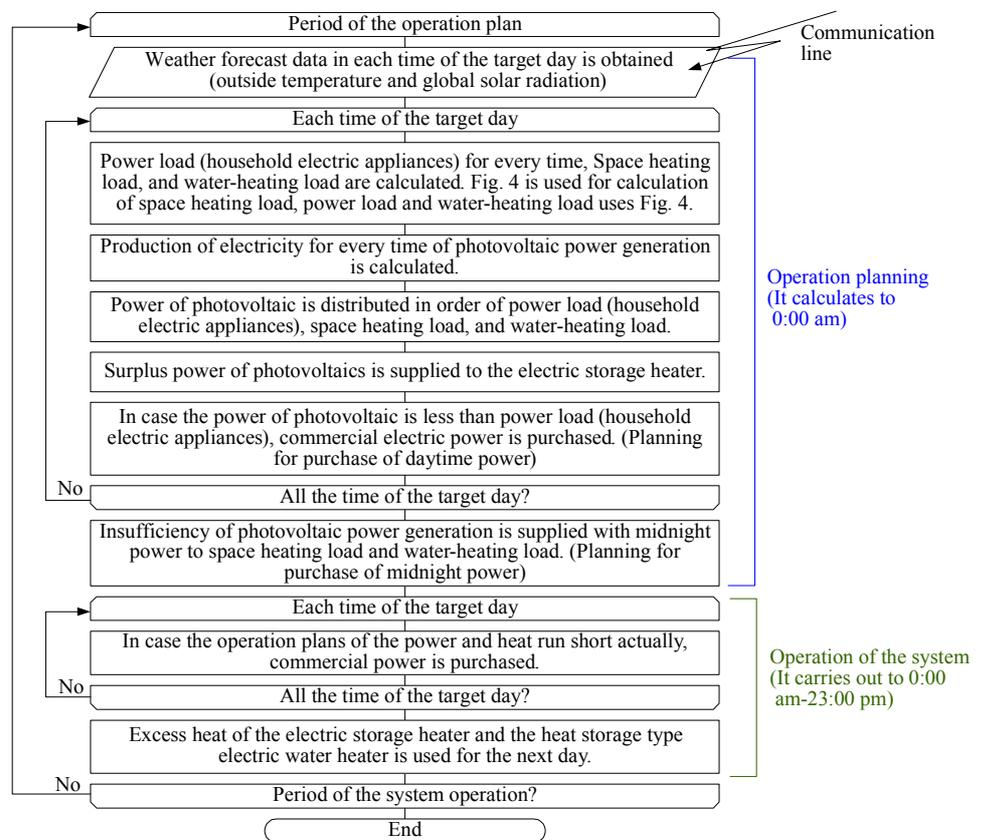
Fig. 8 Control flow of the operation planning and system operation
