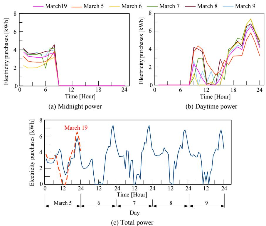
Fig. 12 The amount of electricity purchases. Area of the solar cell module 40 m<sup>2</sup>.
