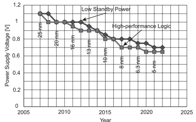
Fig. 1 Power supply voltage trend (ITRS roadmap).
