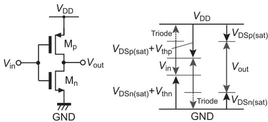
Fig. 3 CMOS inverter (C-INV).
