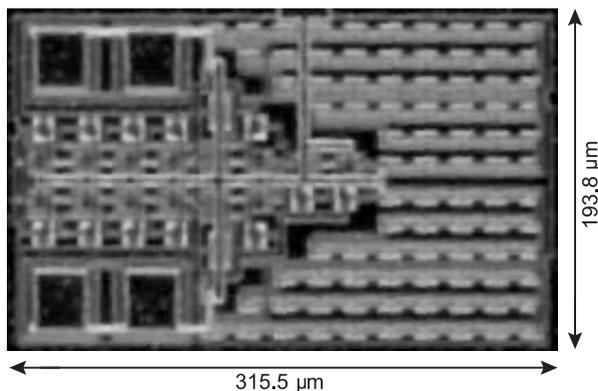
Fig. 10 Chip micrograph of the proposed OTA.
