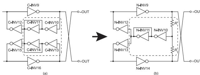
**Fig. 8** Second stage of before (F/B OTA) (a), and after (F/B OTA with resistive common-mode detector) (b).
