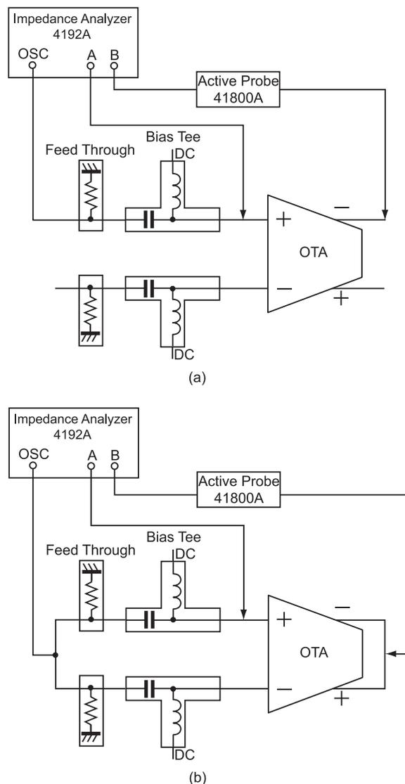
Fig. 11 Measurement setup for OTA of the differential-mode (a), and of the common-mode (b).
