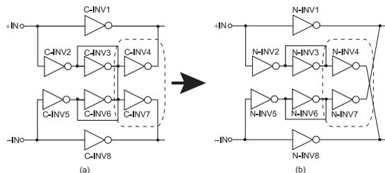
**Fig. 7** First stage of before (F/F OTA) (a), and after (cross F/F OTA) (b).
