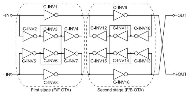
Fig. 5 Circuit configuration of the F/F+F/B OTA.
