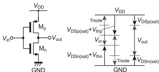
Fig. 3 CMOS inverter (C-INV).
