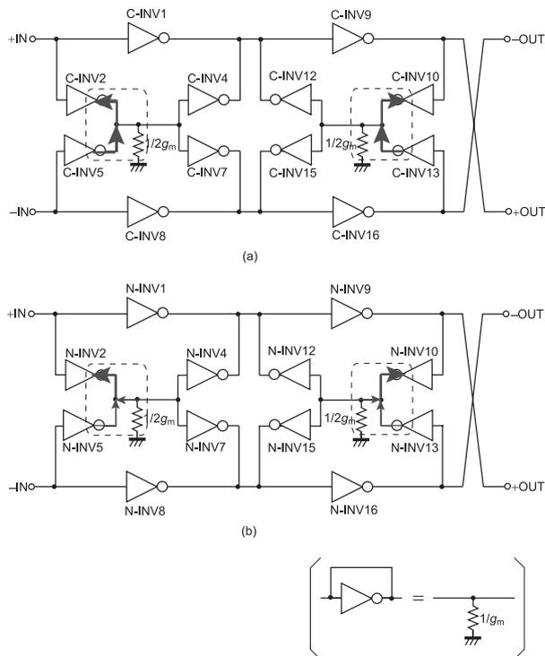
**Fig. 6** Flow of the differential-mode signals of the F/F+F/B OTA using CMOS inverters (a), and using NMOS inverters (b).
