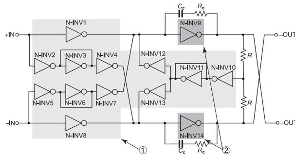
**Fig. 9** Circuit configuration of the proposed OTA.
