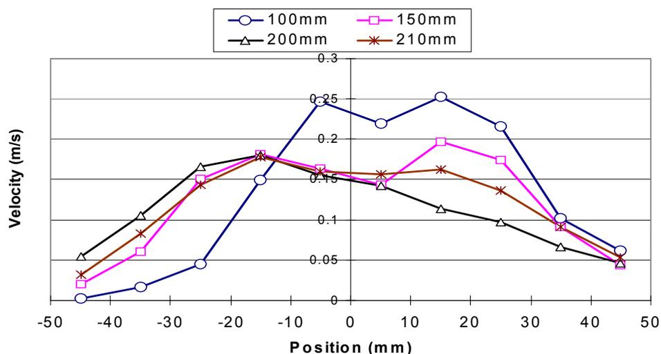
Fig. 11: X-direction velocity for 90-degree and without fire-tube conditions
