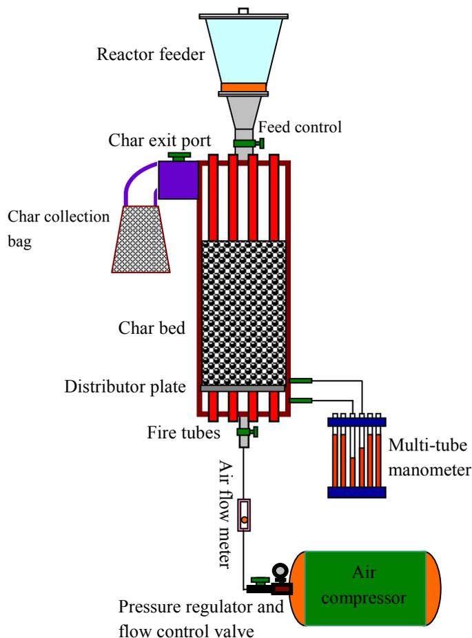
**Fig. 2:** Schematic diagram of a cold model fixed-bed fire-tube heating pyrolysis system for fluid dynamics study to determine char ejection pressure
