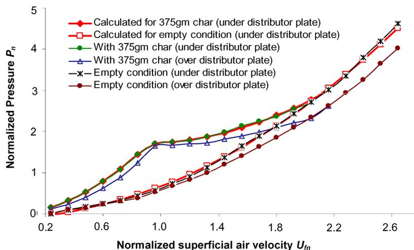
Fig. 3: Pressure difference on upper and lower side of the distributor plate for both of empty and char full conditions with calculated values
