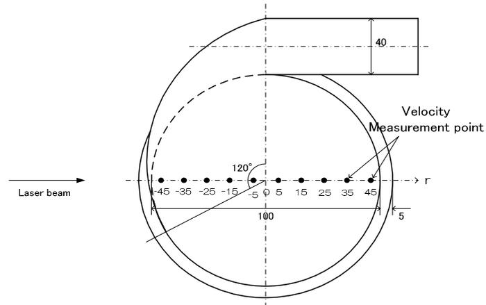
**Fig. 7:** 0-degree position of reactor cylinder for X and Y-velocity component measurements
