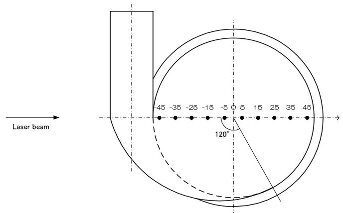
**Fig. 8:** 90-degree position of reactor cylinder for X and Y-velocity component measurements
