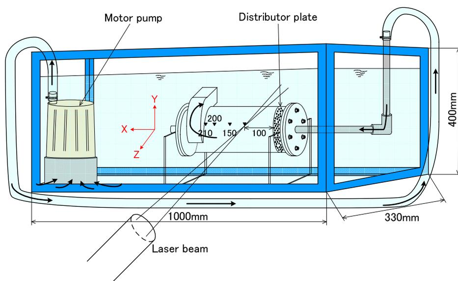
Fig. 6: Schematic diagram of the experimental set-up for LDV measurement
