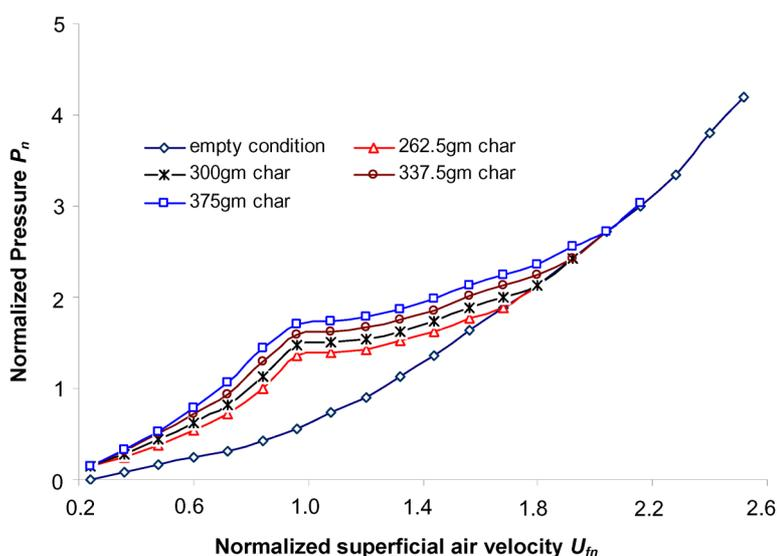
**Fig. 5:** Pressure difference on lower side of the distributor plate,  $P_n$  versus superficial air velocity,  $U_{fn}$  curves for different c
