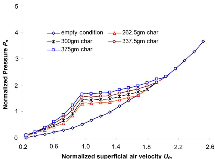
**Fig. 4:** Pressure difference on upper side of the distributor plate,  $P_n$  versus superficial air velocity,  $U_{fn}$  curves for different char weight
