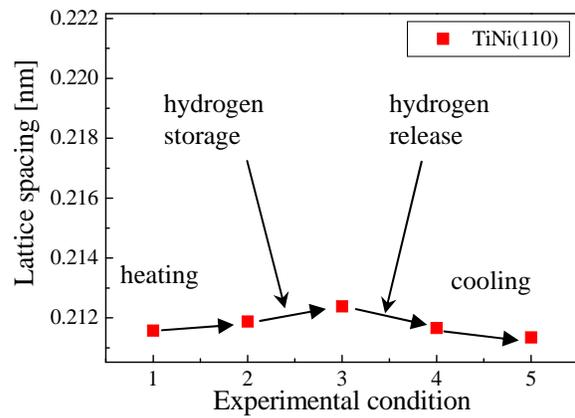
Fig. 8 Change of lattice spacing of TiNi(110) plane due to hydrogen absorption.
