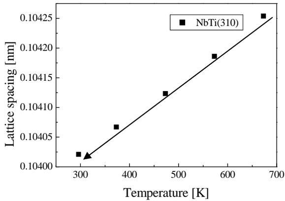
Fig. 3 Change of lattice spacing of NbTi(310) plane with temperature.
