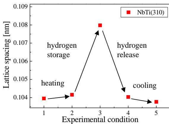
Fig. 7 Change of lattice spacing of NbTi(310) plane due to hydrogen absorption.
