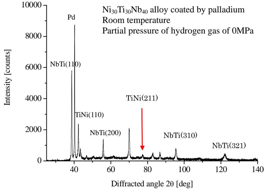
Fig. 2 Diffraction X-ray profile of the as-cast  $\text{Ni}_{30}\text{Ti}_{30}\text{Nb}_{40}$  alloy.
