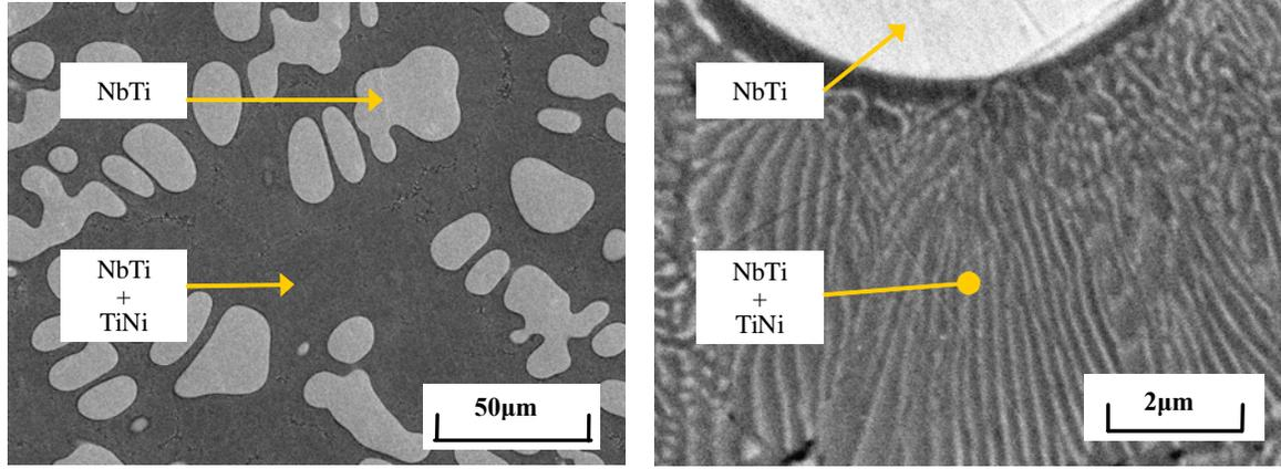
Fig. 1 SEM images of the as-cast  $\text{Ni}_{30}\text{Ti}_{30}\text{Nb}_{40}$  alloy which consists of the primary phase, NbTi, and eutectic phase, TiNi + NbTi.
