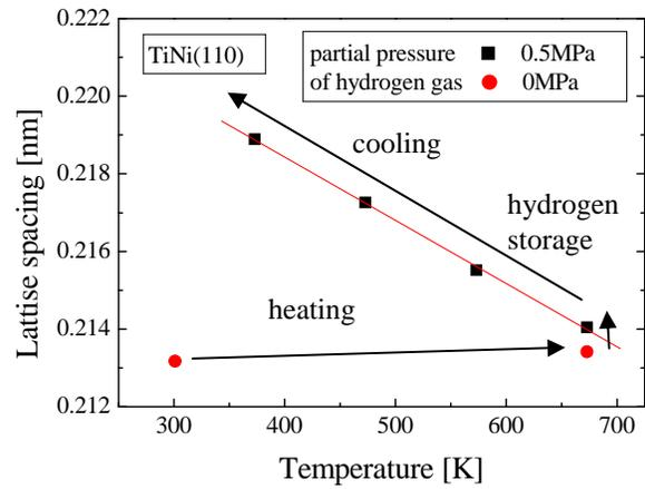
Fig. 6 Change of lattice spacing of TiNi(110) plane with temperature.
