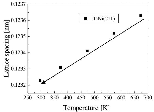
Fig. 4 Change of lattice spacing of TiNi(211) plane with temperature.
