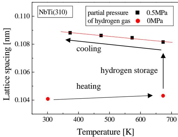
Fig. 5 Change of lattice spacing of NbTi(310) plane with temperature.
