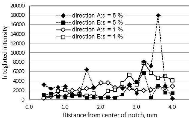
Fig.9 Integrated intensity of Al 220 diffraction profile.
