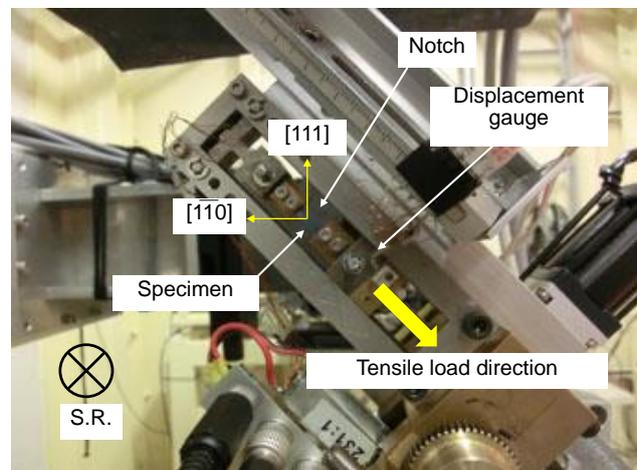
Fig.2 Compact tension equipment for strain measurement using synchrotron white X-ray.
