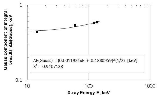
Fig.10 Gauss component of integral breadth of instrumental function in the measurement system.
