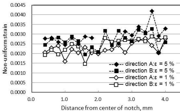
Fig.11 Distribution of non-uniform strain calculated by using Al220 diffraction profile.
