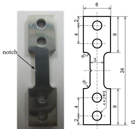
Fig.1 Specimen configuration for tensile test.
