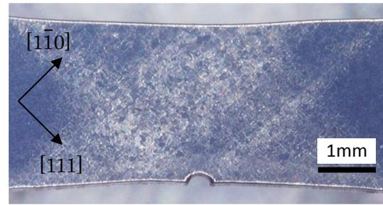
Fig.13 Distribution of slip band near notch of aluminum single crystal at applied strains of  $\epsilon=5\%$ .
