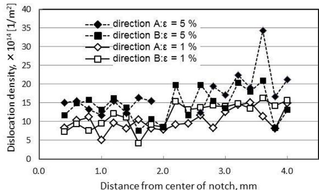
Fig.12 Distribution of dislocation density calculated by using Al 220 diffraction profile.
