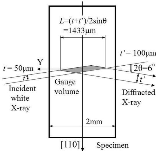
Fig.3 Schematic diagram of gauge volume using transmission diffracted X-ray.
