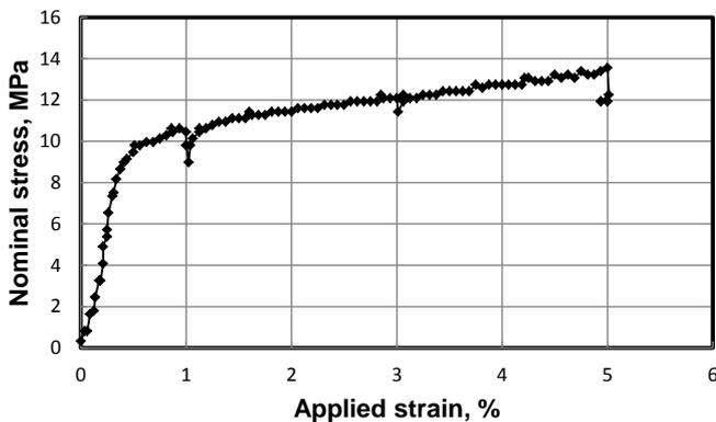
Fig.5 Stress-strain diagram and measurement points of one-side notched Al single crystal specimen.
