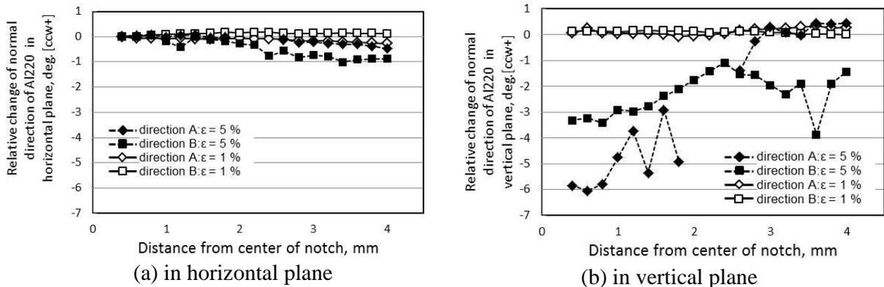
Fig.8 Distribution of relative rotation angle of normal direction of diffraction plane of Al220.
