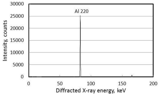
Fig.4 Diffracted X-ray profile of Al single crystal.
