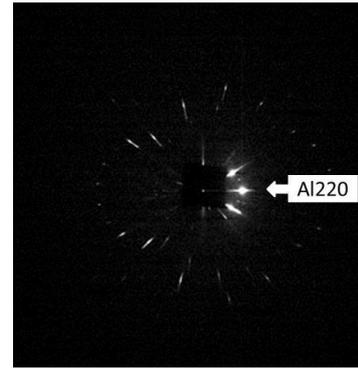
Fig.7 Transmission SR Laue diffraction pattern of Al single crystal by flat panel sensor.
