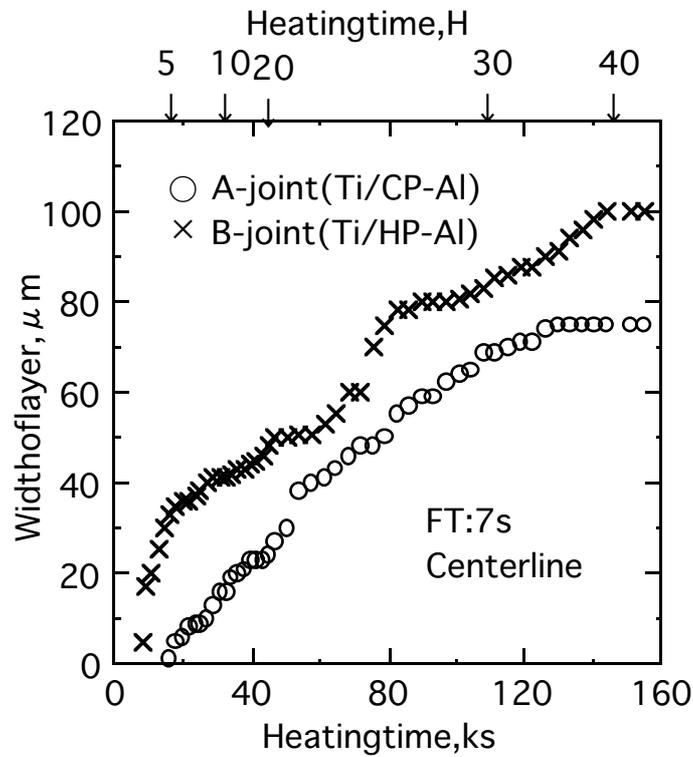
Fig.6 Relationship between heating time and layer growth at centreline of A and B joints welded with FT of 7 s, using linear scale for heating time.
