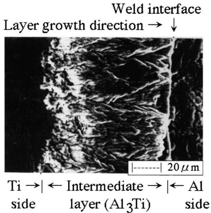
Fig.3 Example of microstructure of interlayer at interface of pure Ti – commercially pure Al friction weld heated at 580uC for 200 h (optical).
