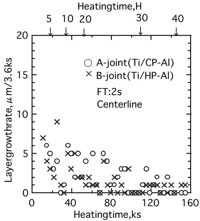
Fig.7 Relationship between increase in layer thickness per 3.6 ks (1 h) and heating time at centreline of A joint welded with FT of 2 s.
