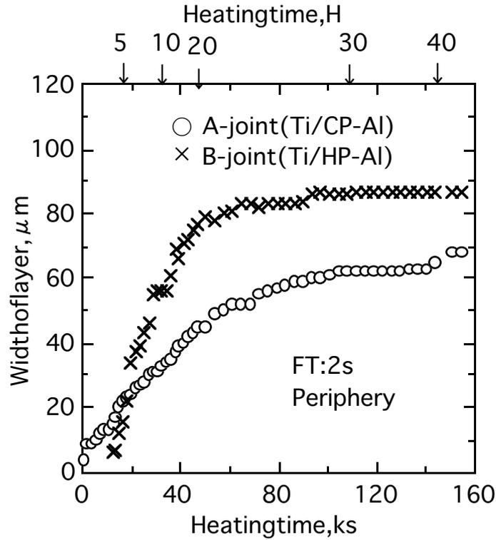
Fig.5 Relationship between heating time and layer growth at periphery of A and B joints welded with FT of 2 s, using linear scale for heating time.
