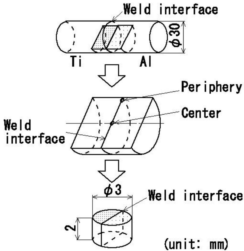
Fig.1 Specimen preparation method for in situ observation.
