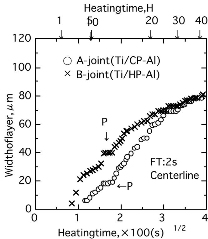
Fig.4 Relationship between heating time and layer width at interface of centreline region of pure Ti – commercially pure Al joint (A joint) and pure Ti – highly pure Al joint (B joint) welded with friction time (FT) of 2 s: results are shown using a linear scale and b square root scale for heating time (horizontal axis).
