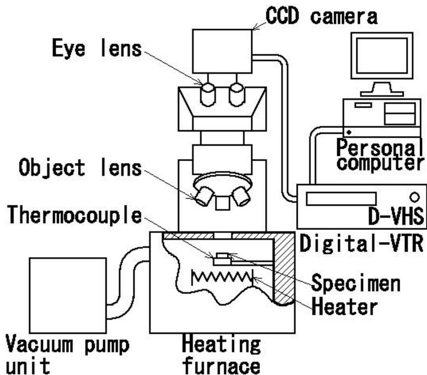
Fig.2 Schematic illustration of in situ observation system
