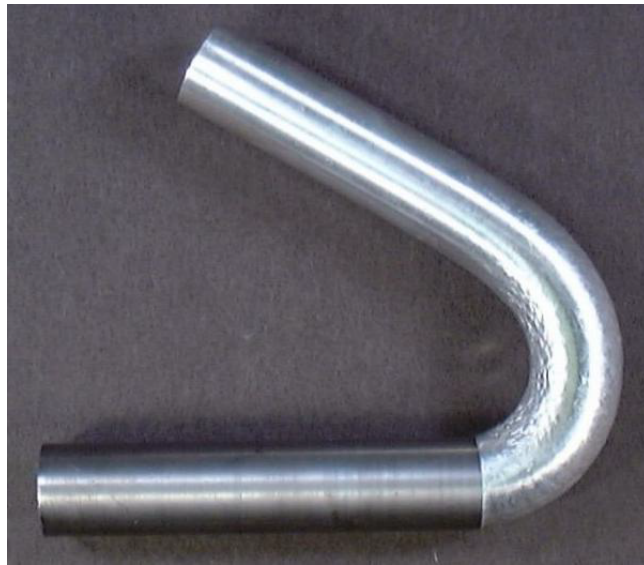
Fig.10 Appearance of bend test specimens in as-welded condition after test.
