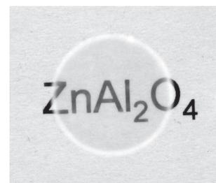
Fig. 3. Transparent ZA ceramics annealed at 1100°C for 3 h in air after sintering. The sample with diameter 10 mm and thickness 1.3 mm is 24 mm above the text.
