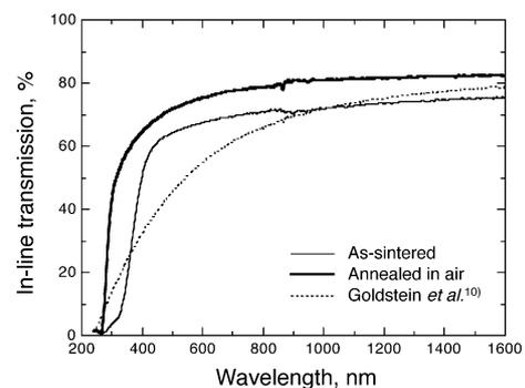
Fig. 4. In-line transmission after sintering and annealing. The measured transmission was converted for a thickness of 1 mm.
