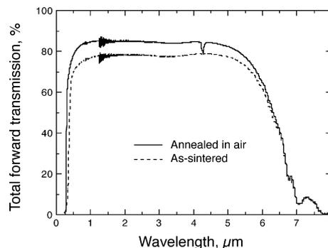
Fig. 6. Total forward transmission after sintering and annealing.
