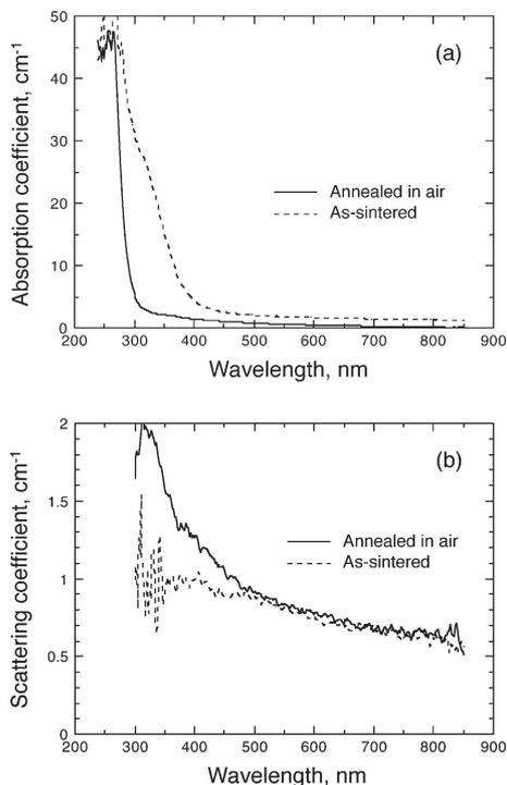
Fig. 5. (a) Absorption and (b) scattering coefficient before and after annealing.
