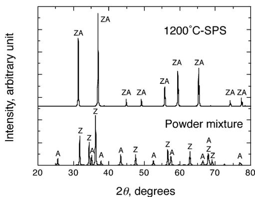
Fig. 1. XRD pattern for powder mixture and sintered body. Z, A and ZA represents ZnO, Al<sub>2</sub>O<sub>3</sub> and ZnAl<sub>2</sub>O<sub>4</sub>, respectively.
