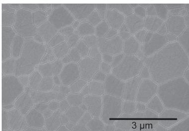
Fig. 2. Microstructure of sintered zinc aluminate.
