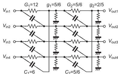
Fig. 9 Realized RC PF for example 7.
