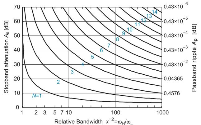
Fig. 5 Relation between number of sections, attenuation and bandwidth.
