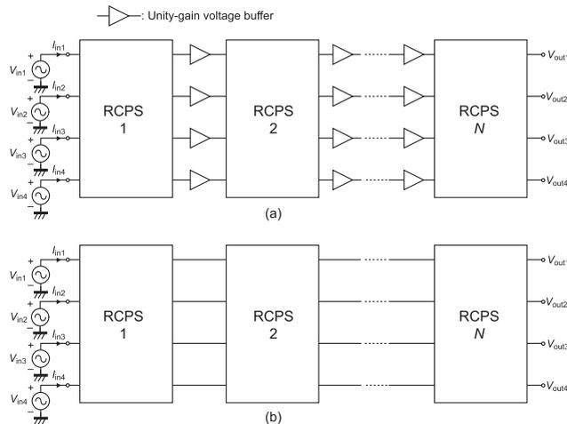
**Fig. 3** Multi-stage RC PF with (a), and without (b) interstage voltage buffers.
