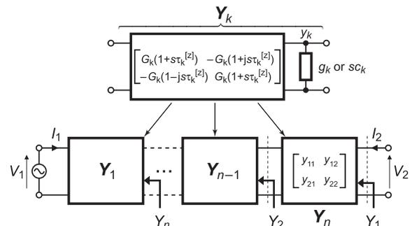
Fig. 8 Cascade synthesis procedure.
