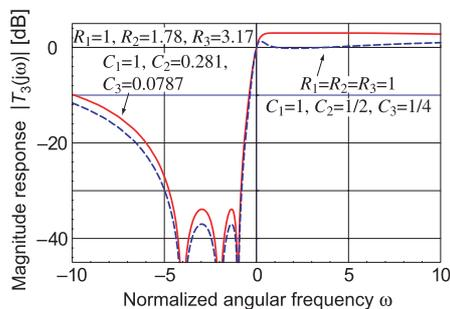
**Fig. 4** Example magnitude response of 3-stage RC PF.
