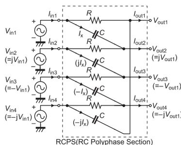
Fig. 1 Single-stage four-phase RCPF (RCPS).
