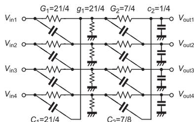
Fig. 10 Realized RC PF for example 8.
