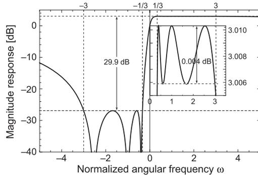
**Fig. 7** Magnitude response of transformed equal ripple RCPF.
