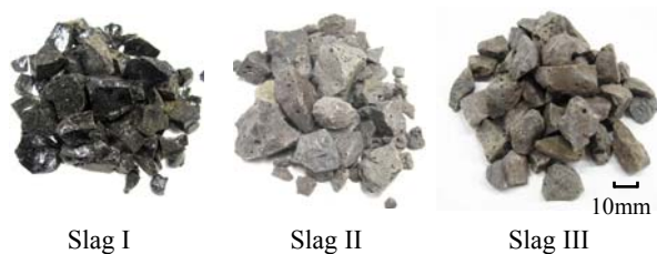
Fig.1 Sewage sludge molten slag coarse aggregate.
