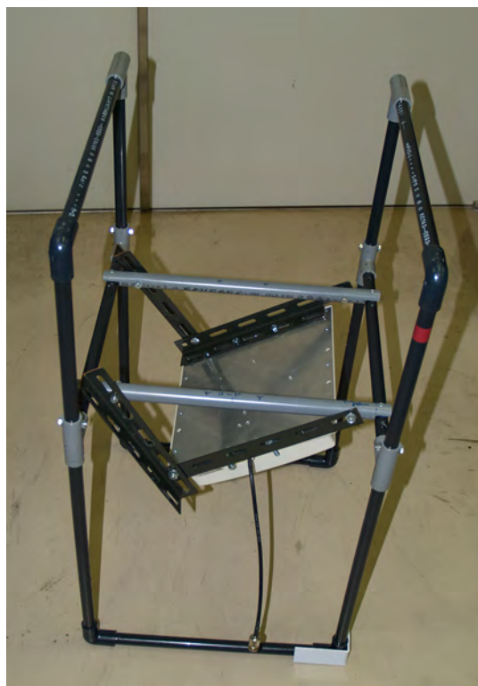
Fig.5 UHF RF-ID antenna fixed on PVC frame with 30 degree.
