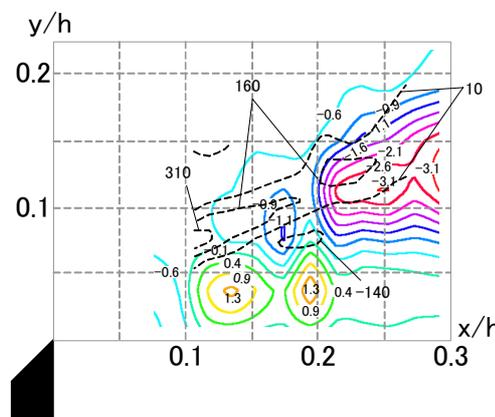
Fig.10 Reynolds shear stress distribution and vorticity decay rate (black dotted lines)
