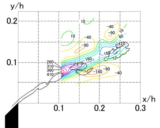
Fig.9 Vorticity decay rate distribution with visualization photo
