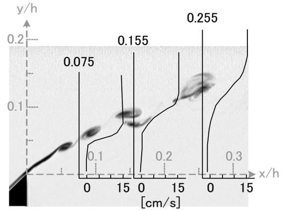
Fig.3 Visualization photo and velocity distribution at each  $x/h$  position
