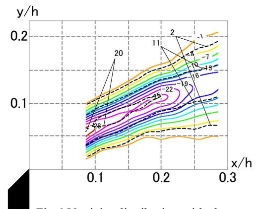
Fig.6 Vorticity distribution with shear strain rate (black dotted lines)
