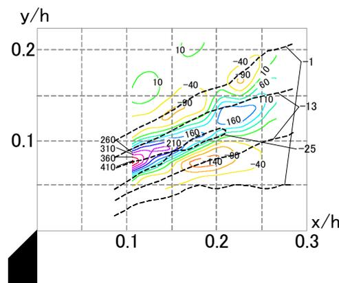
Fig.7 Vorticity decay rate distribution with vorticity (black dotted lines)
