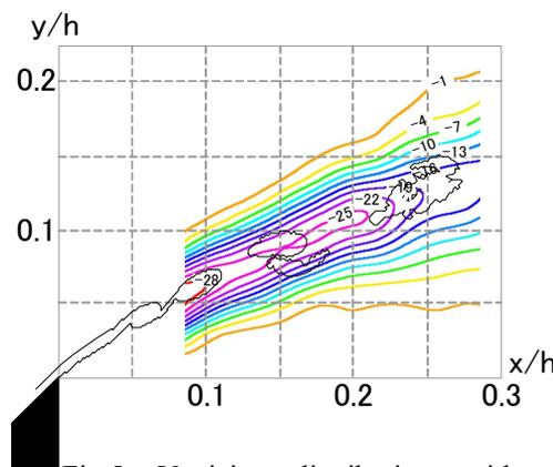
Fig.5 Vorticity distribution with outlines of visualization photo
