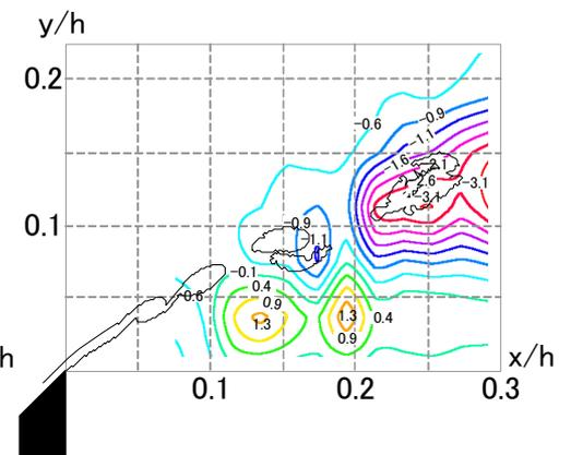
Fig.11 Reynolds shear stress distribution and visualization photo
