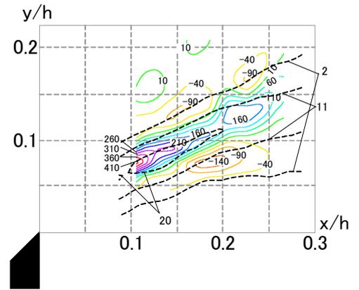
Fig.8 Vorticity decay rate distribution with shear strain rate (black dotted lines)
