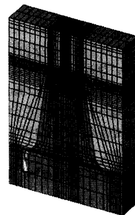
Fig.2 Finite element meshing employed for the numerical analysis.
