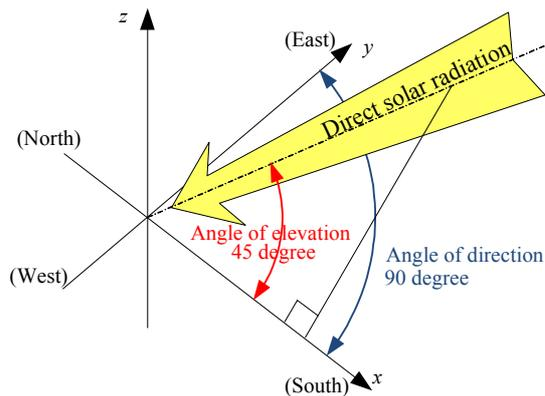
Fig. 7 The coordinate system used in the case analysis
