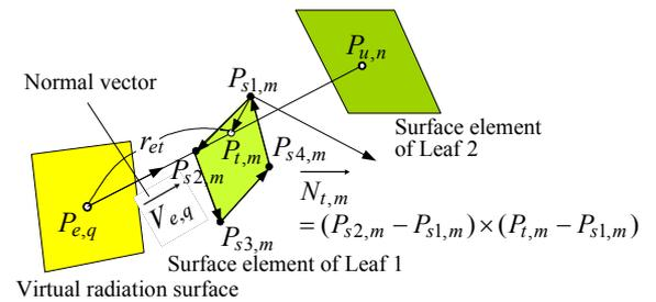
Fig. 8 Interrupt check of light quanta
