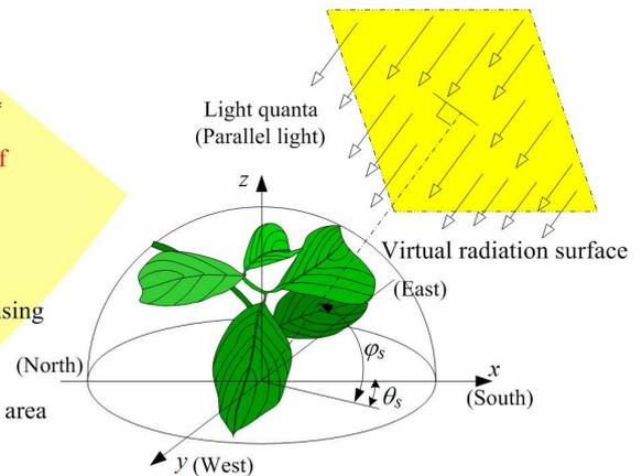
Fig. 2 Space coordinate of a virtual radiation surface
