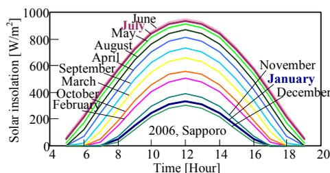
Fig. 13 Insolation of the level surface
