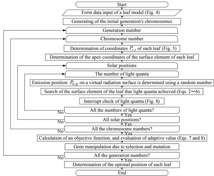
Fig. 10 Calculation flow of LAPS
