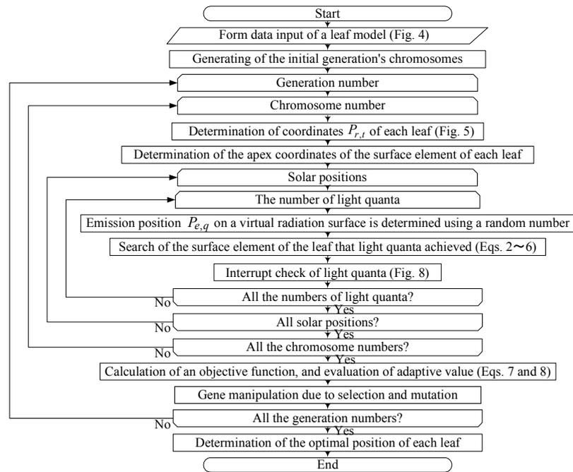
Fig. 10 Calculation flow of LAPS
