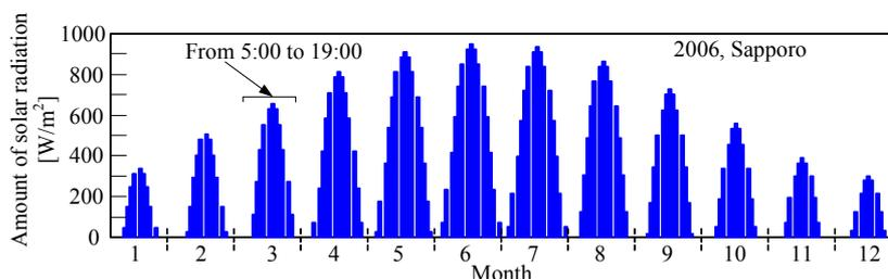
Fig. 12 The amount of solar radiation on the horizontal plane
