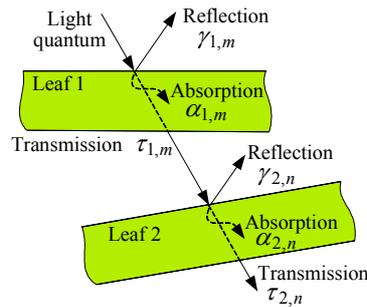
Fig. 7 Optical system model
