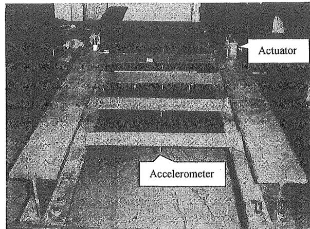
Fig. 2 Accelerometers and actuator positions
