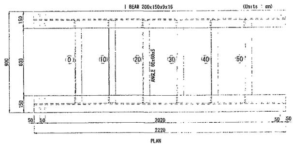
Fig. 1 Specimen dimensions
