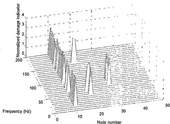
Fig. 7 DIM applied to experimental data for Case 3, normalized damage indicator value at each frequency.
