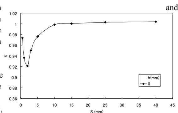
Fig. 6 Control effect for depth  $h=0\text{mm}$
