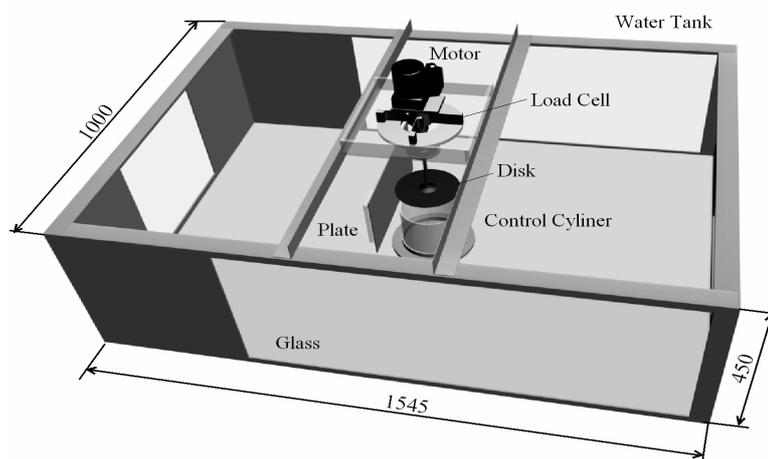
Fig. 1 Schematic diagram of the experimental arrangement
