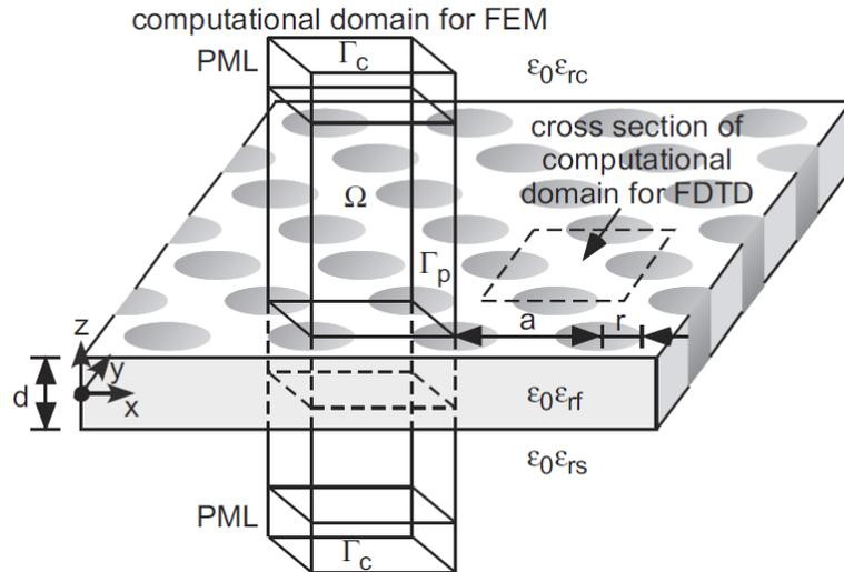
Fig. 1. Geometry of photonic crystal slab.
