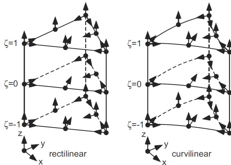
**Fig. 2.** Rectilinear and curvilinear mixed-interpolation-type triangular-prism elements.
