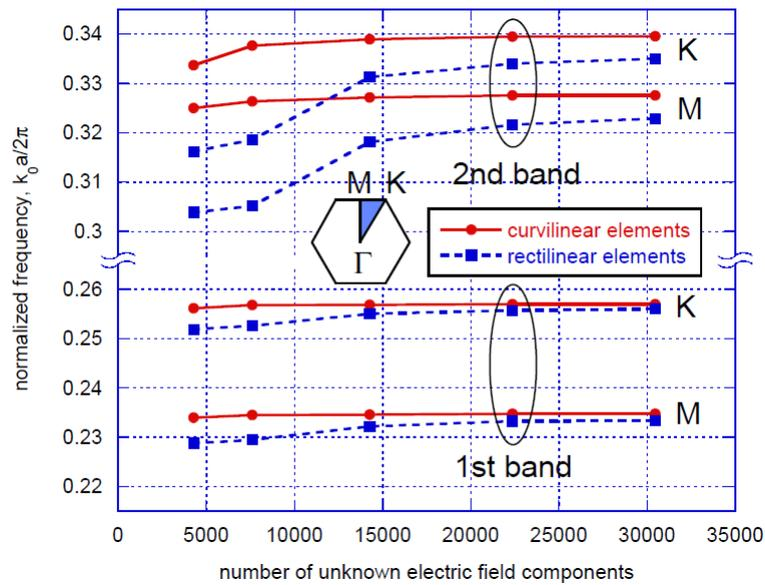
(a) Convergence of the solution against the number of the unknown electric field components.
