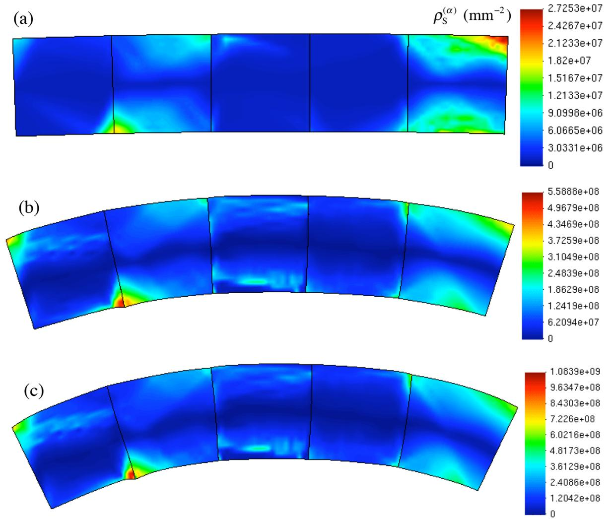
**Figure 5.** Deformed configurations of the foil ( $H = 12.5 \mu\text{m}$ ) and contours of SSD densities on primary slip system at (a)  $\theta H / L = 0.013$ , (b)  $\theta H / L = 0.123$ , and (c)  $\theta H / L = 0.178$ .
