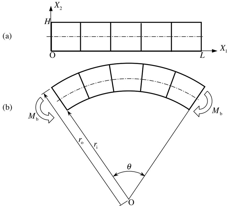
**Figure 1.** Problem formulation of pure bending of a thin foil with grain size being about equal to the thickness.
