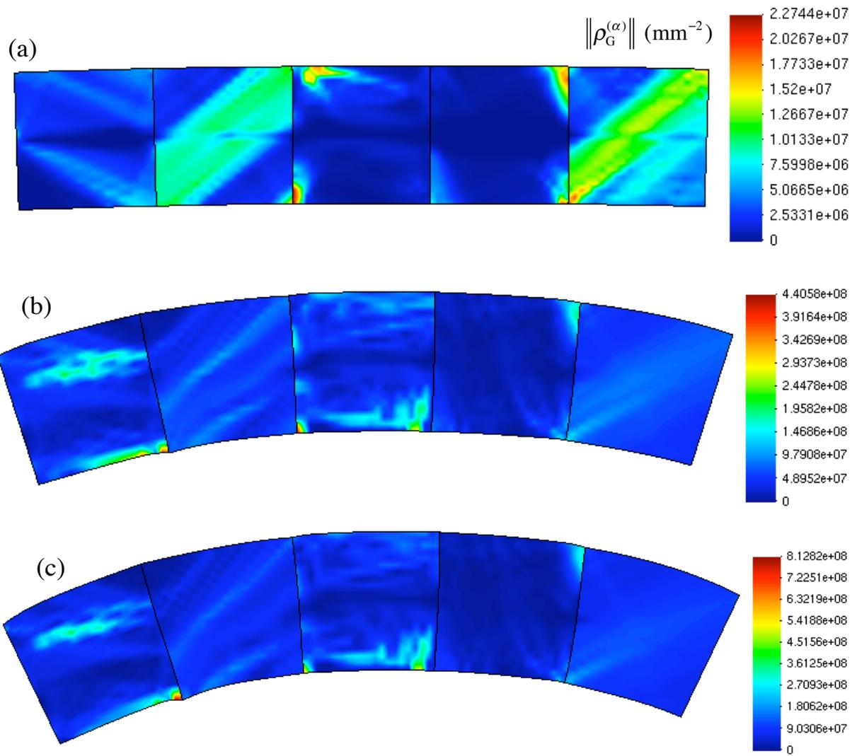
**Figure 4.** Deformed configurations of the foil ( $H = 12.5 \mu\text{m}$ ) and contours of GND densities on primary slip system at (a)  $\theta H / L = 0.013$ , (b)  $\theta H / L = 0.123$ , and (c)  $\theta H / L = 0.178$ .
