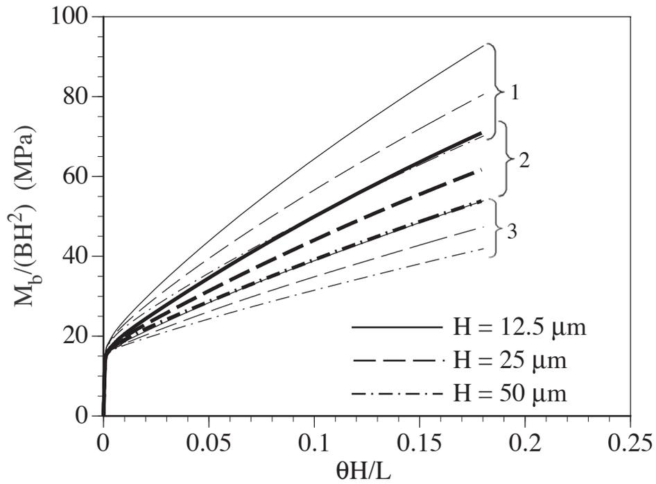
**Figure 2.** Appearance of size effect on computed curves of bending moment versus bending angle for three sets of randomly chosen grain orientations.
