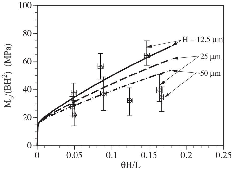
**Figure 3.** Comparison of computed curves of bending moment versus bending angle to experimental results of Stölken and Evans (1998).
