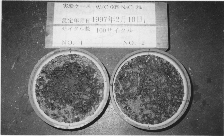
Photo-2 Result of substantiation test with solution of NaCl 3% wt. (w/c=60%)
