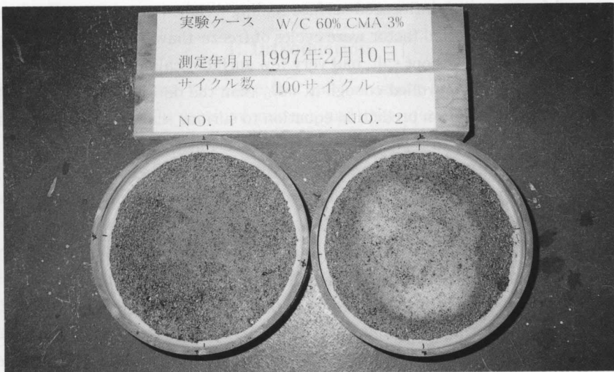
Photo-1 Result of substantiation test with solution of CMA 3% wt. (w/c=60%)
