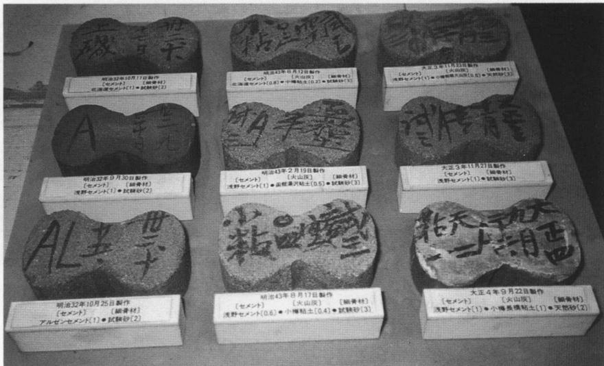
Photo.-2 Specimen of mortar (Maximum length : 80 mm, minimum width : 20 mm, thickness : 22.2 mm)
