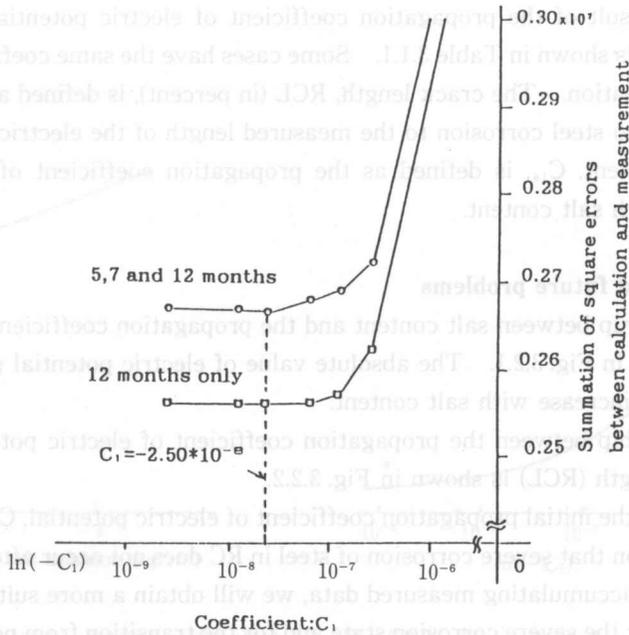
Fig. 3.1.1 Relationship between  $C_1$  and the summed squared errors between calculation and measurement
