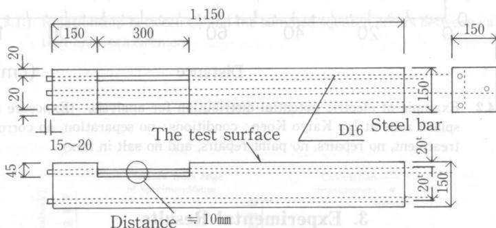
Fig. 2.4.1 The layout of measured specimens
