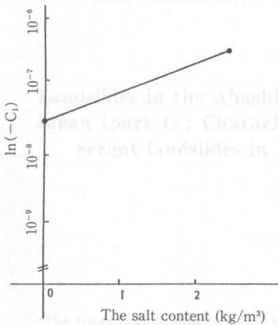
Fig. 3.2.1 The relationship between salt content and propagation coefficient of electric potential ( $C_1$ )
