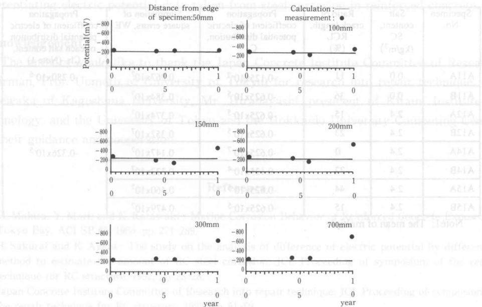
Fig. 3.1.2 Relationship between calculated and measured electric potential gradients
