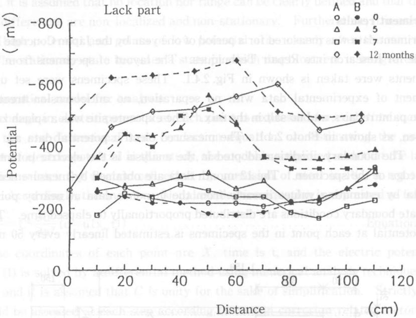
Fig. 2.4.2 Example of electric potential distribution for analysis. (Exposure site: splash zone at Izu Kaiyo Koen; conditions: no separation, no corrosion treatment, no repairs, no paint repairs, and no salt in mix)
