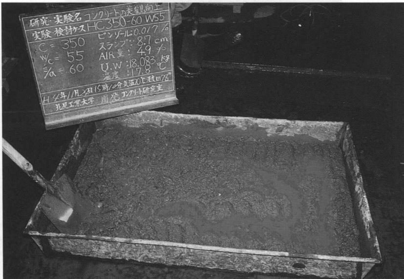
Photo 1 Fresh concrete before adding color admixture
