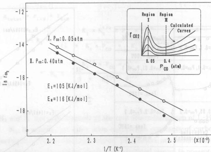
Fig. 5 Comparison of Arrhenius plots of  $r_{CO_2}$  at regions I and II.
