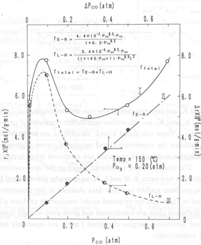
**Fig. 1** Interpretation of the anomalous steady state rate data as a function of  $P_{CO}$ .
