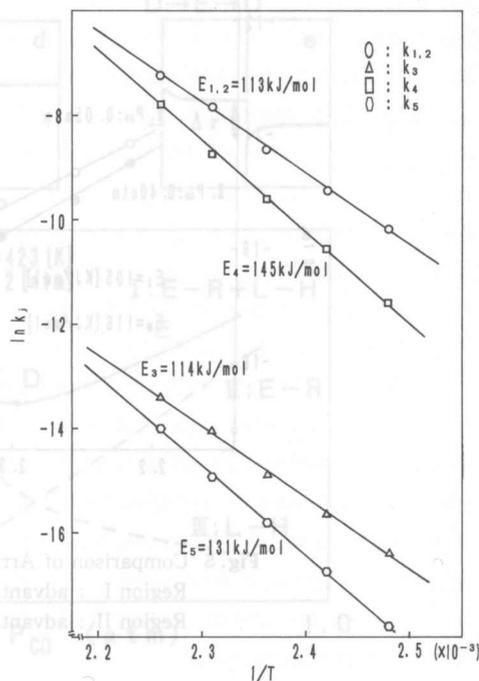
Fig. 3 Arrhenius plots of  $k_j$  evaluated by the computer simulation.
