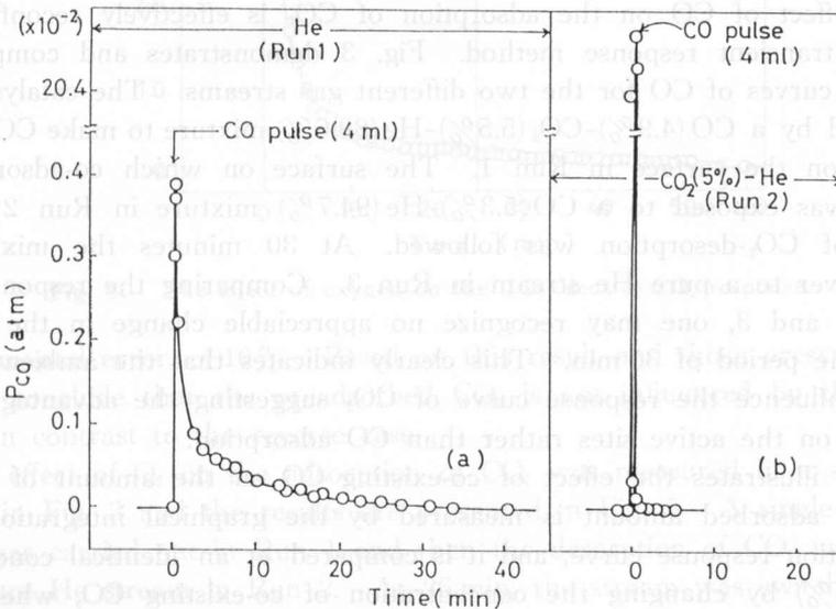
Fig. 2. Chromatographic responses of CO and CO<sub>2</sub> due to the pulse technique.
