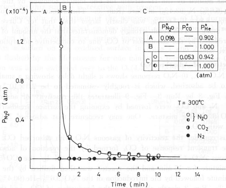
Fig. 9. Reactivity of adsorbed  $N_2O$  with  $CO$ .
