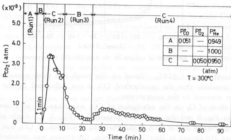
Fig. 6. Reactivity of adsorbed CO.
