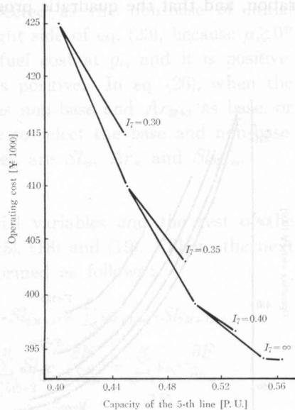
Fig. 4. Operating cost for  $I_5$  ( $Y=210$ ,  $I_1=1.1$ ,  $I_4=0.45$ ).
