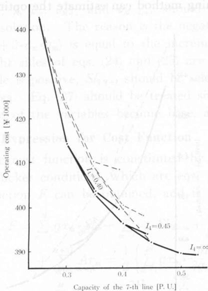
Fig. 3. Operating cost for  $I_7$  ( $Y=210$ ,  $I_1=1.1$ ).
