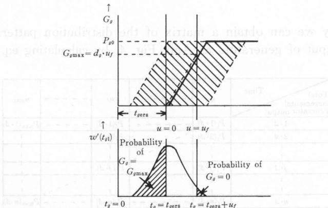
App. Fig. 2. Distribution of  $t_g$  and generator output at  $u_f$ .
