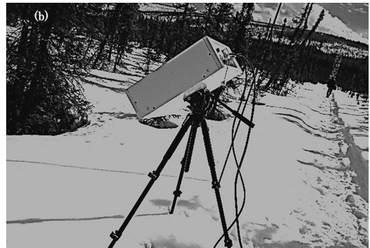
Fig. 2 Microwave radiometer MMRS2 used in this study. (a) Device construction, (b) the image shows field experiment at the Poker Flat Research Range (PFRR).
