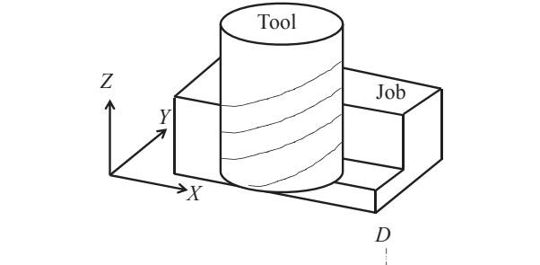
**Fig. 3.** Basic cutting conditions of an end milling operation.
