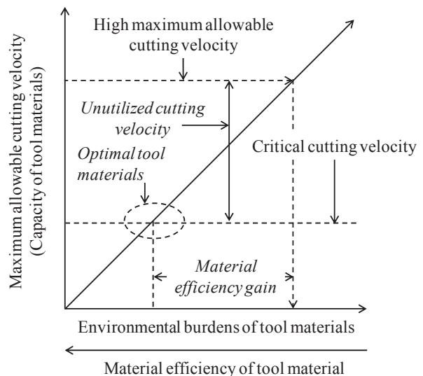
**Fig. 7.** Cutting tool development using the strategy of high cutting velocity.
