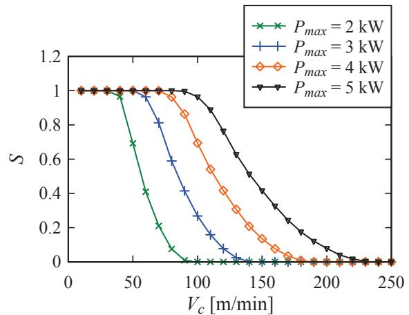
**Fig. 6.** Total rate of success versus cutting velocity for different machine capacities.
