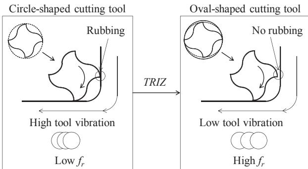
**Fig. 9.** Applying TRIZ in developing a milling tool.
