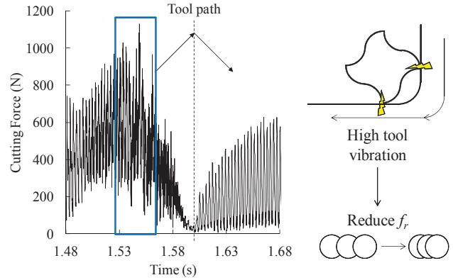
**Fig. 8.** Consequences when a cutting tool passes a sharp corner.
