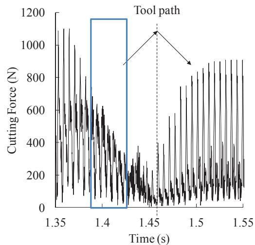
**Fig. 10.** Cutting force underlying an oval-shaped milling tool.
