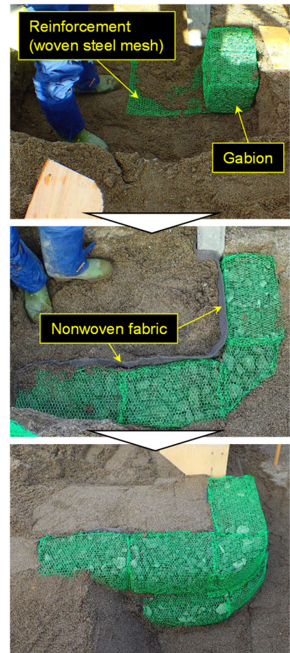
Fig.10 Construction process of model gabion-reinforced soil wall.
