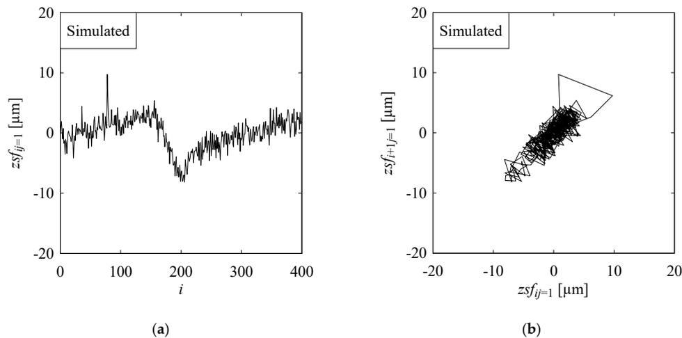
Figure 11. Outcomes of the Monte Carlo simulation-based SC associated with the semantic modeling-based MC: (a) simulated surface heights; (b) return map of (a).
