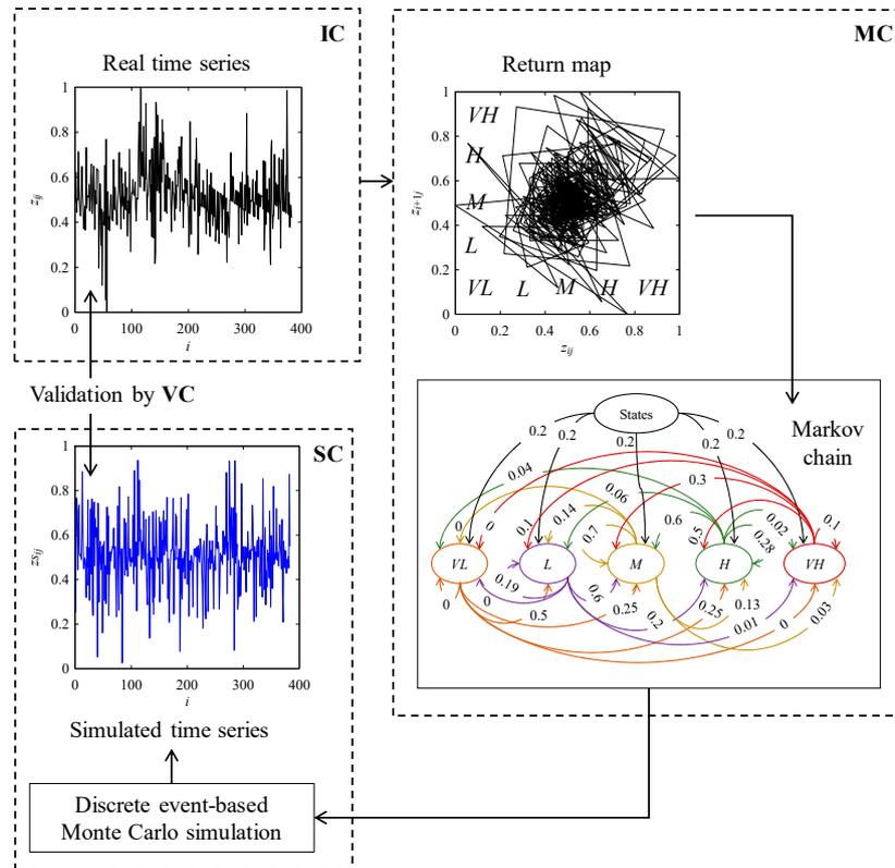
**Figure 5.** Outlining phenomenon twin construction of surface roughness using the Markov chain-based modeling approach [17].
