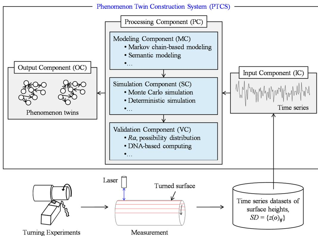
Figure 3. Outlining the phenomenon twin construction of surface roughness.
