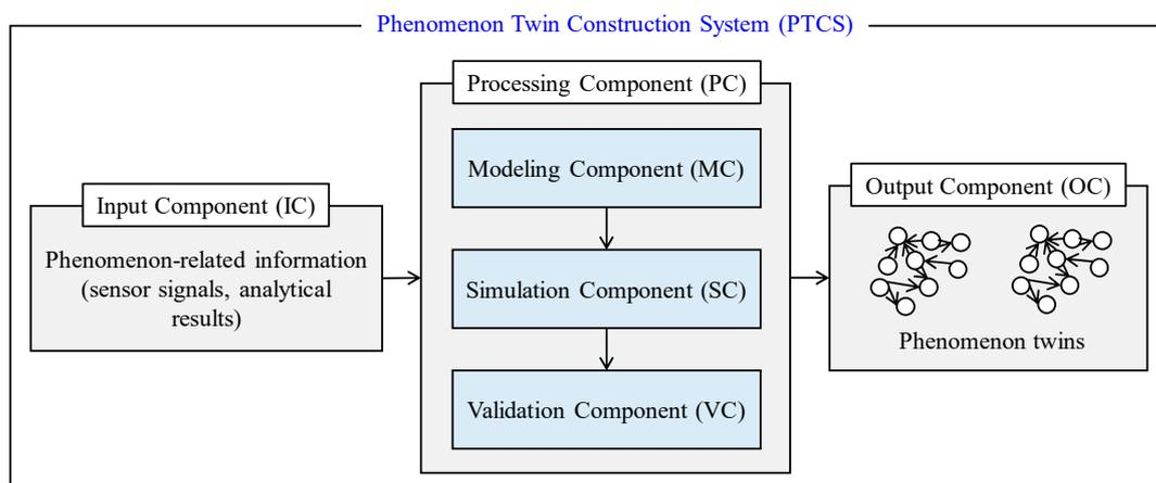
**Figure 2.** Proposed architecture of Phenomenon Twin Construction System (PTCS).
