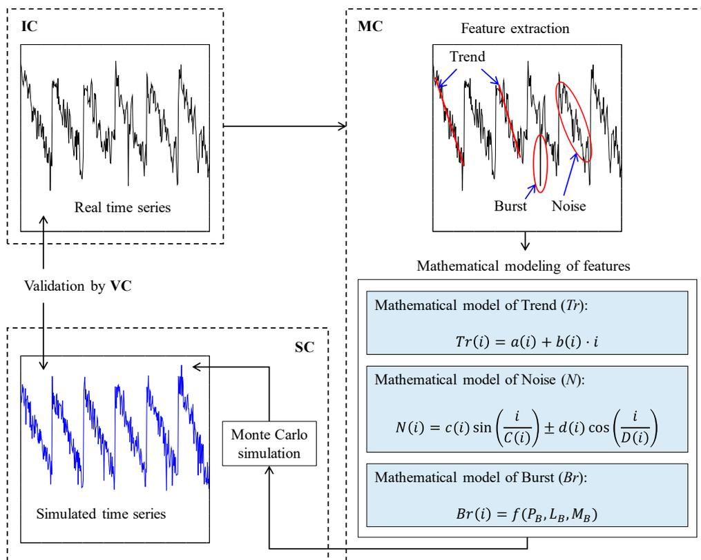
**Figure 9.** Outlining phenomenon twin construction of surface roughness using the semantic modeling approach [16].
