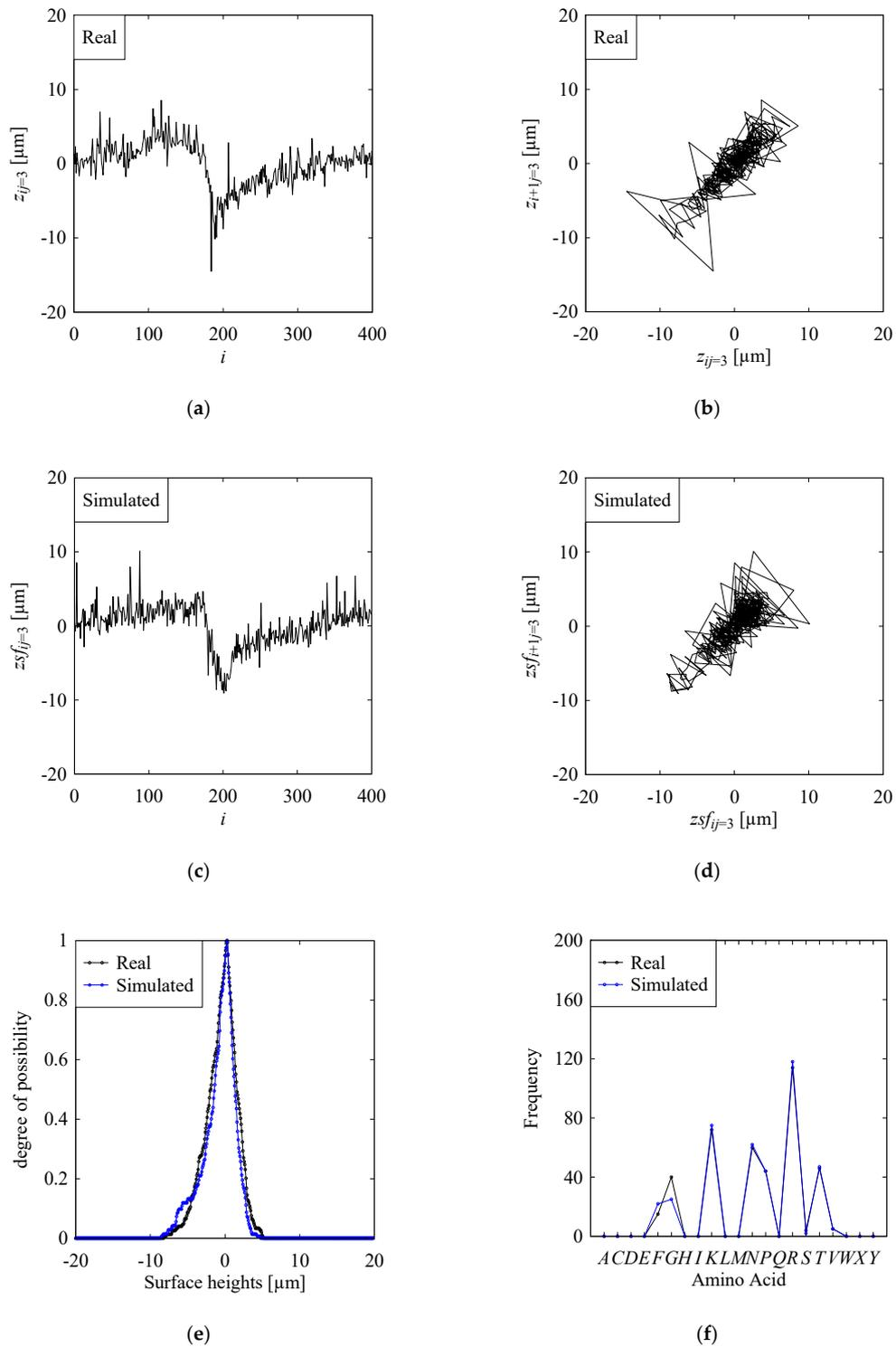
Figure A3. Outcomes of SC and VC corresponding to the semantic modeling-based MC for  $z_{ij=3}$ : (a) real surface heights; (b) return map of (a); (c) simulated surface heights; (d) return map of (c); (e) possibility distribution; (f) DNA-based computing.
