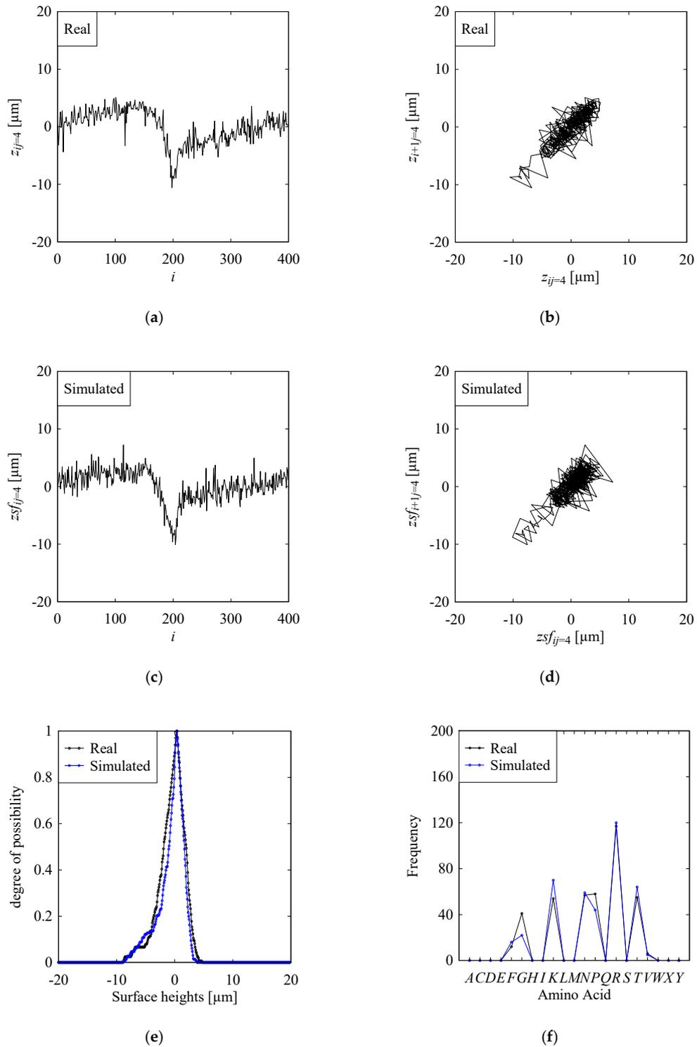
**Figure A4.** Outcomes of SC and VC corresponding to the semantic modeling-based MC for  $z_{ij=4}$ : (a) real surface heights; (b) return map of (a); (c) simulated surface heights; (d) return map of (c); (e) possibility distribution; (f) DNA-based computing.
