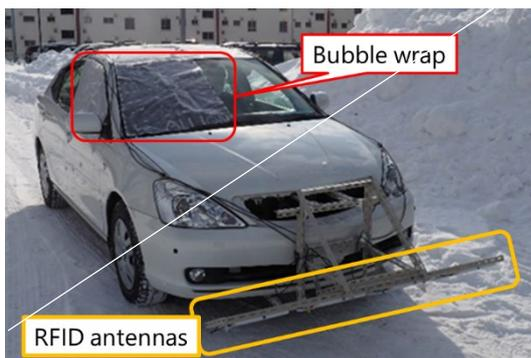
Fig. 5 The driving experiment vehicle
