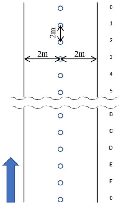
**Fig. 3** Driving experiment road (○: RFID tag installed point)
