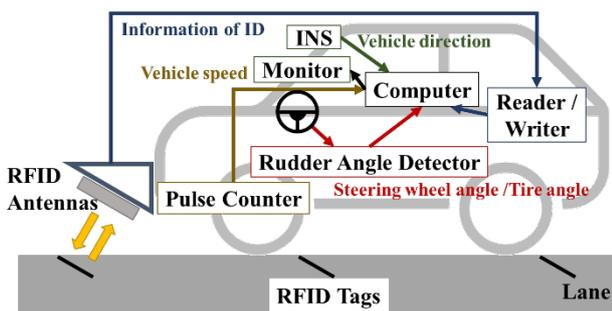
Fig. 1 The schematic of vehicle navigation system
