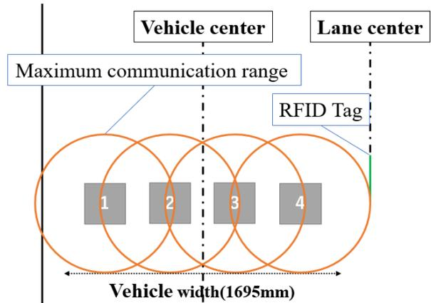
Fig. 2 Position of 4 RFID antennas and a RFID tag
