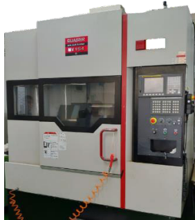
Fig. 1 Digital control milling machine (MV154-C)
