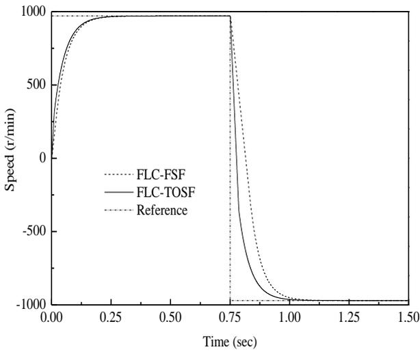
(c) Speed transient from 0 r/min to 970 r/min followed by speed reversion from 970 r/min to -970 r/min at 0.75 sec.
