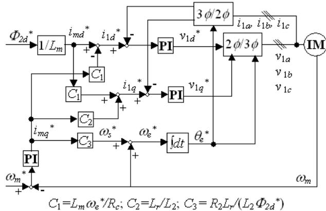
Fig. 2. Control structure of IM taking core loss into account based on PI controller
