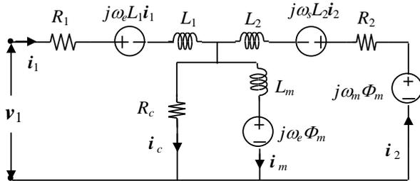
Fig. 1. Equivalent circuit of IM taking core loss into account.
