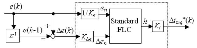
Fig. 3 Control structure of a standard FLC.
