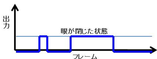
Fig. 9 Changes in the iris detection status during blinking and slow closing/opening.
