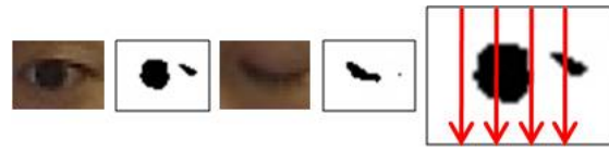
Fig. 5 Left: Binarization, two examples of image E and image B combinations. Right: Scan direction to judge the opening/closing status, indexed by a longest part of red lines traversing black areas.
