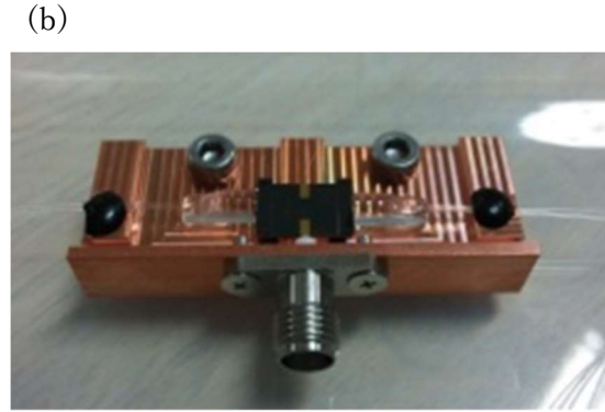
Figure 2. (a) Schematic of fibre-coupled module and (b) fabricated module.
