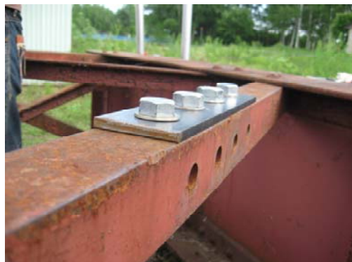
Photo 6 Damage D2 by removing all bolts at vertical splice
