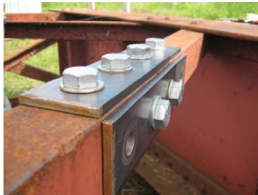
Photo 5 Damage D1 by removing outside 2 bolts at vertical splice
