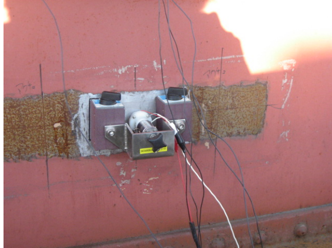
Photo 2 Actuator set on center of web plate in the middle of G1 girder
