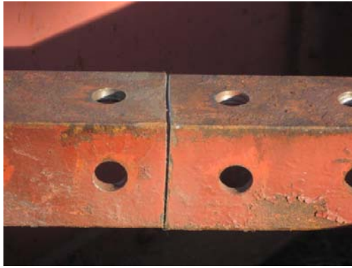
Photo 3 Full cut of cross section of lateral member L2
