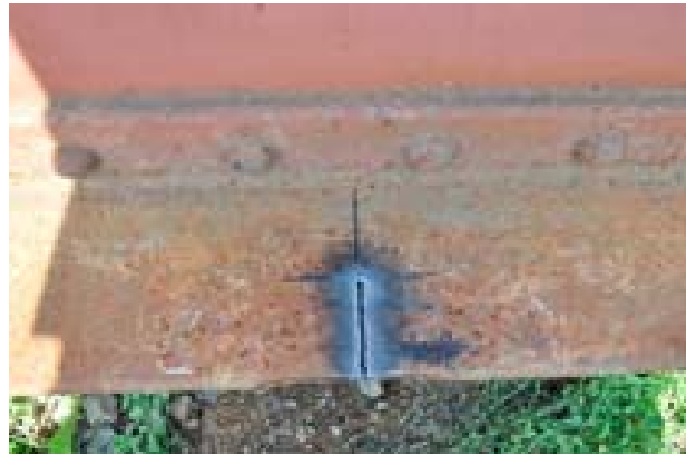
Photo 3 Artificial Crack of Case 1 by one fourth of flange width
