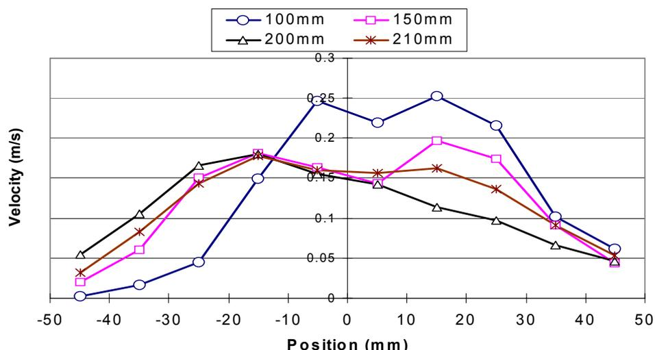
Fig. 11: X-direction velocity for 90-degree and without fire-tube conditions
