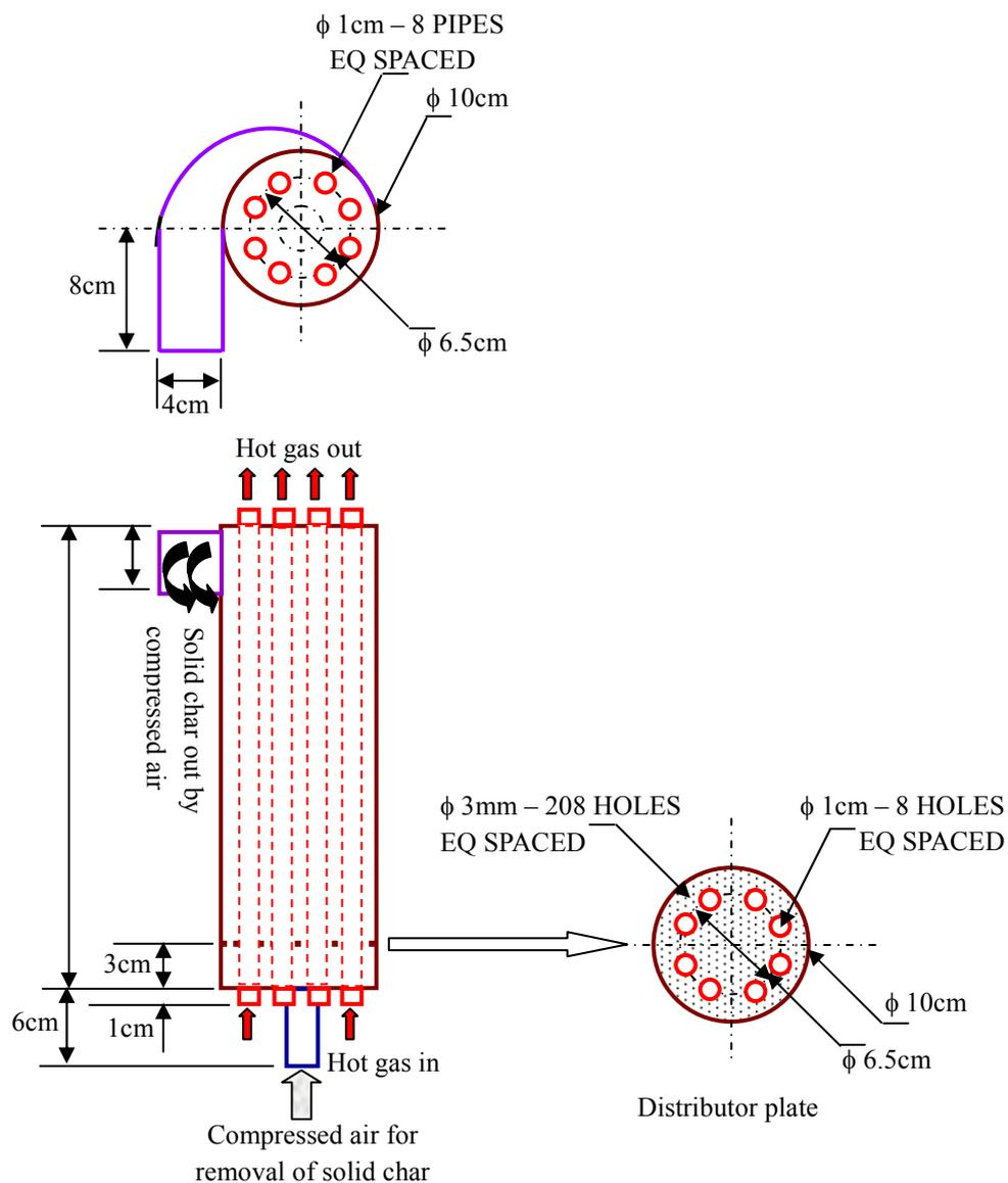
Fig. 1: Detail drawing of the cold model of a fire-tube reactor chamber
