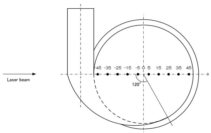
**Fig. 8:** 90-degree position of reactor cylinder for X and Y-velocity component measurements
