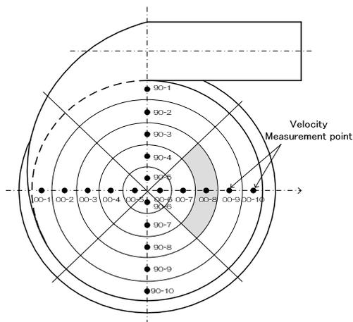
**Fig. 9:** Representation of method adopted for flux calculation
