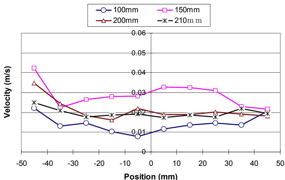
Fig. 14: Y-direction velocity for 0-degree and with fire-tube conditions
