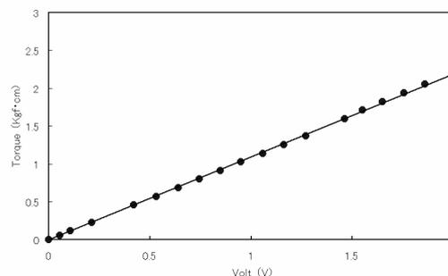
Fig. 4 Strain gauge output voltage against torque
