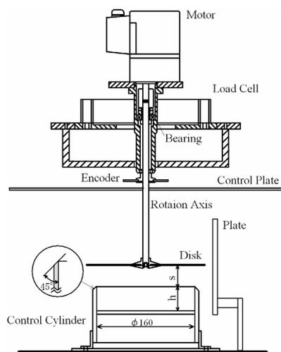
Fig. 2 Experimental set-up of rotating disk
